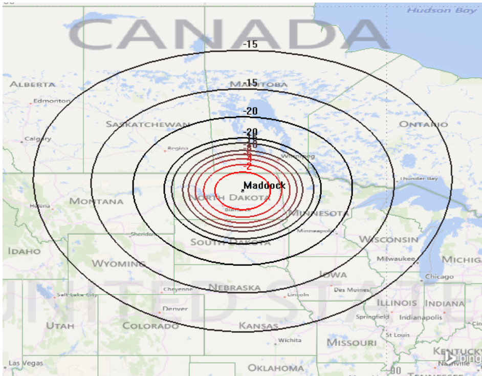
Figure 8 X-band helical antenna gain contour at 410 km altitude over Maddock, ND ground station.
