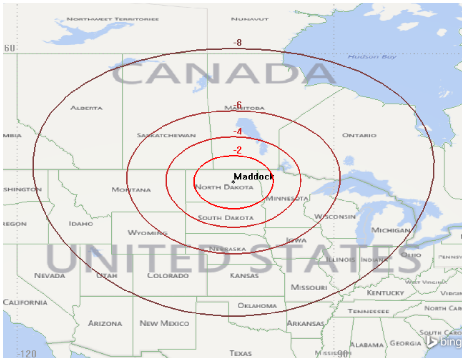
Figure 10 X-band patch antenna gain contour at 410 km altitude over Maddock, ND ground station. 25
