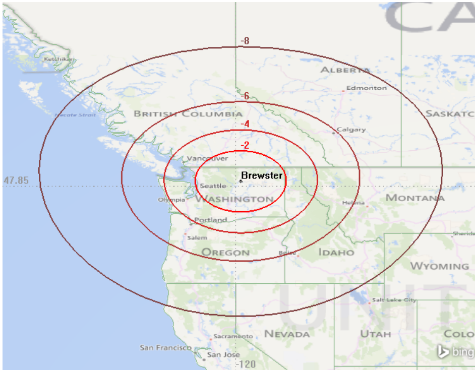
Figure 3 X-band patch antenna gain contour at 300km altitude over Brewster, WA ground station. 22
