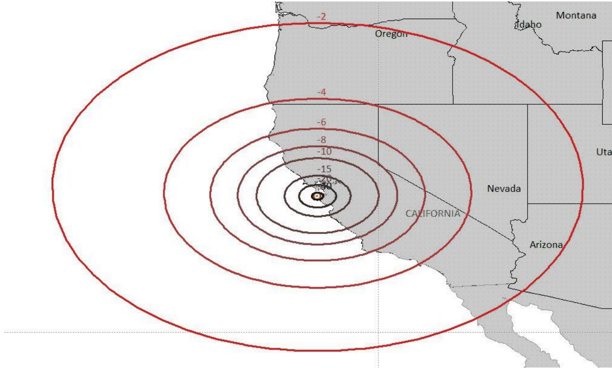
Figure 14 UHF monopole antenna gain contour at 620 km altitude over Half Moon Bay, CA ground station.
