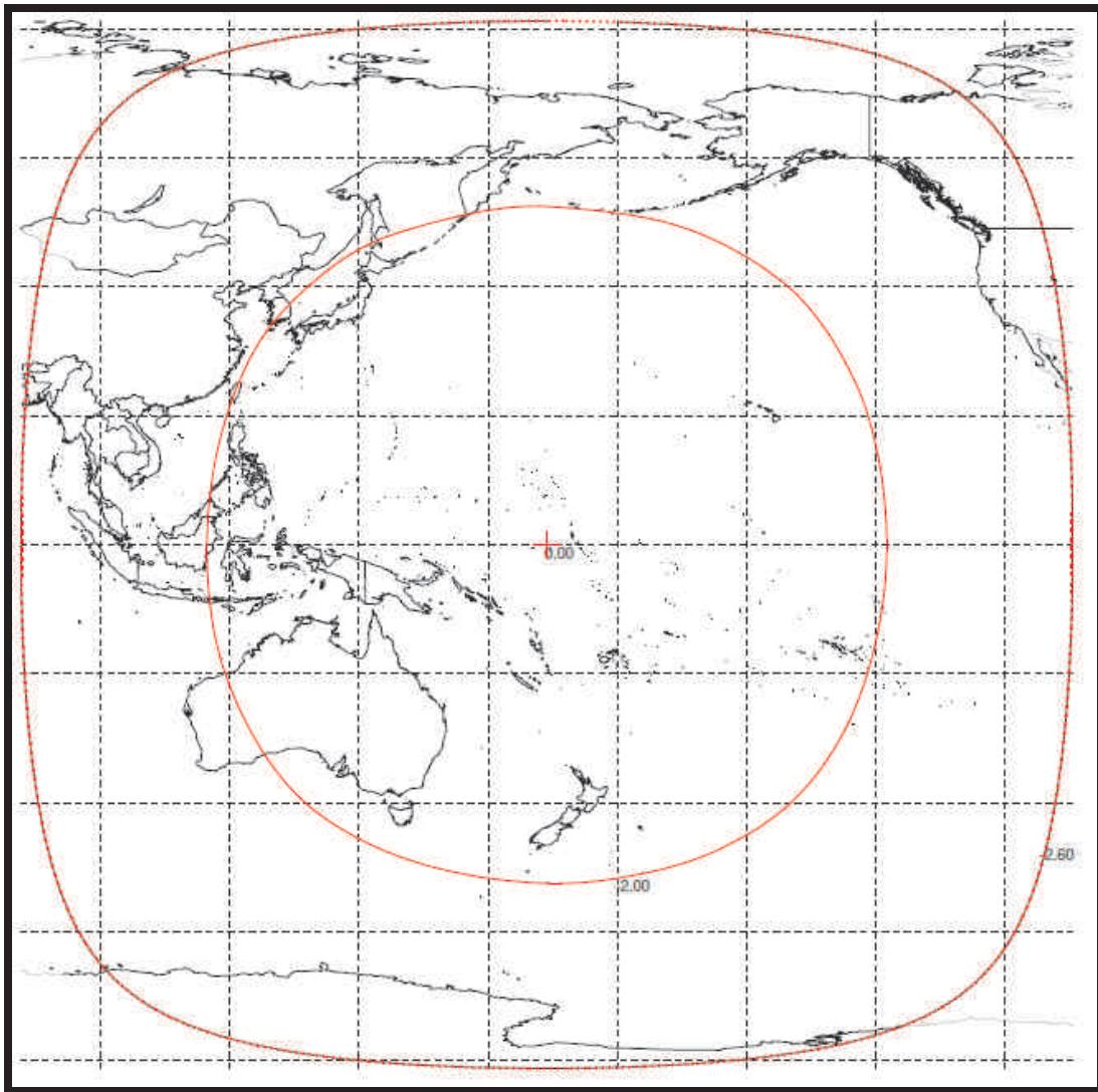
**Exhibit 2-12: Telemetry Downlink Beam [Global Horn Antenna]**
