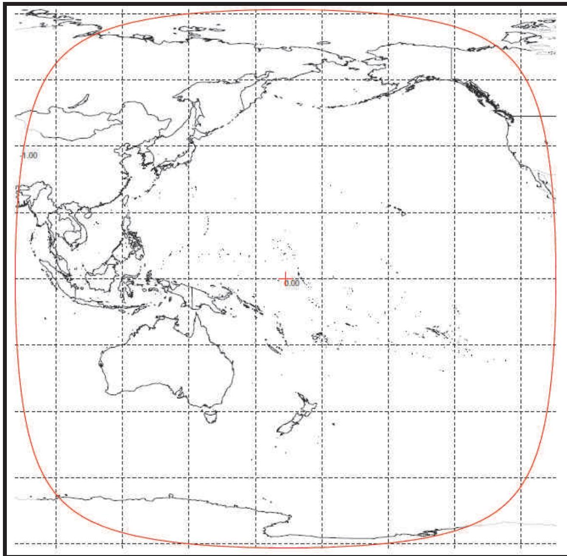
**Exhibit 2-11: Telemetry Downlink Beam [Global Horn Antenna]**
