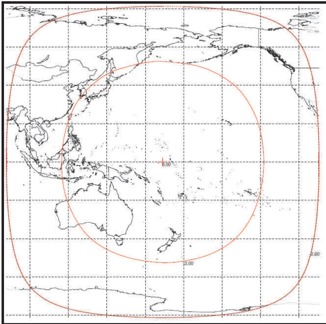
**Exhibit 2-13: Telemetry Downlink Beam [+Z / -Z Antennas]**
