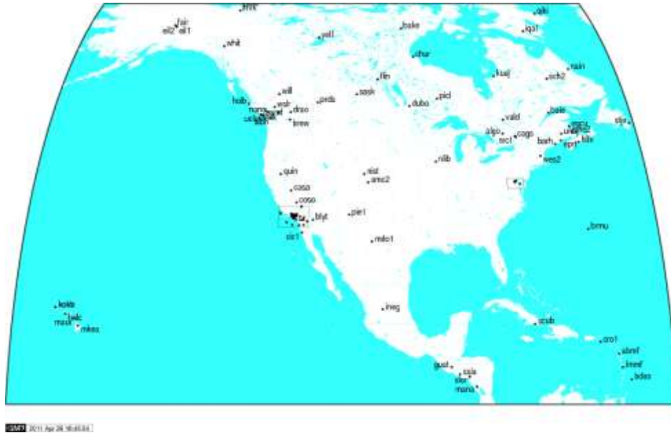
Figure 6-6. Locations of GPS Receivers of the International GNSS Service (IGS). There are 58 receivers in CONUS. The IGS collects, archives, and distributes GPS data for a wide range of applications and experiments (e.g. earth rotation, ionospheric maps, GPS/GLONASS ephemeris).
