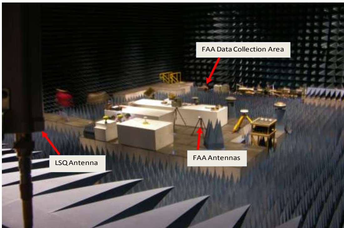
Figure 5-25. Chamber View Looking down from LSQ Antenna
