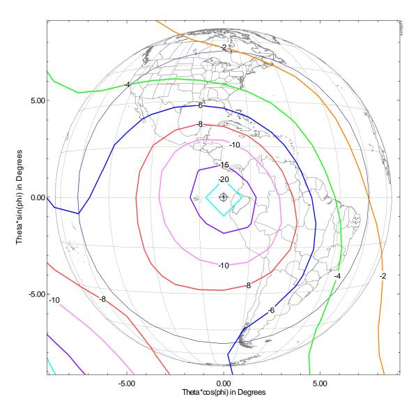
GSO Satellite at 83W Transmit and Receive Beacon Beam - Xpol
