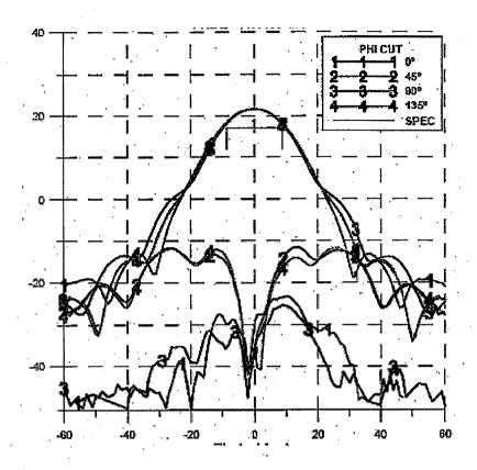
Note: Y-axis is gain (dBi) and X-axis is angle (degrees)
