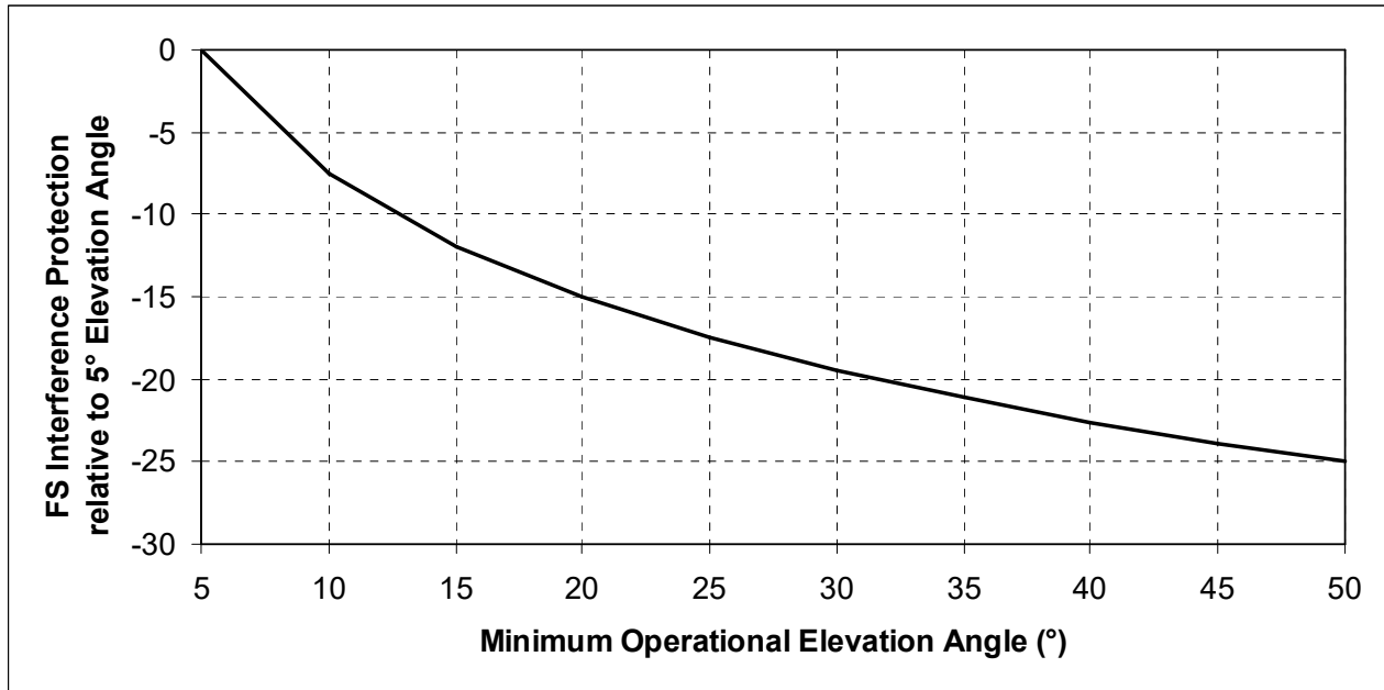
Figure 3.13.4-1: Interference Protection with Respect to FS Systems as a Function of the Minimum Operational Angle of Separation between the Active Virtual Geo Satellite and the GSO Arc
