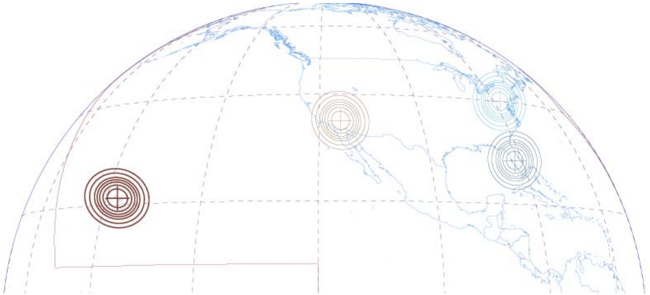
Figure 2-3. Spot Beams (28, 31, 48, 50) Antenna Gain Contours (Contours shown -2dB,-4dB,-6dB,-8dB,-10dB and -20dB)
