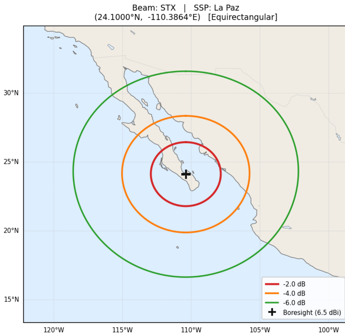
Figure 149. STX Antenna Beam Projection over La Paz from Orbit altitude of 350 km
