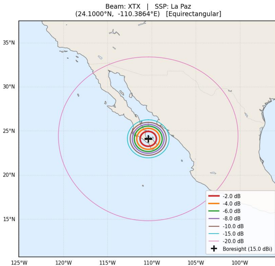
Figure 196. XTX Antenna Beam Projection over La Paz from Orbit altitude of 510 km
