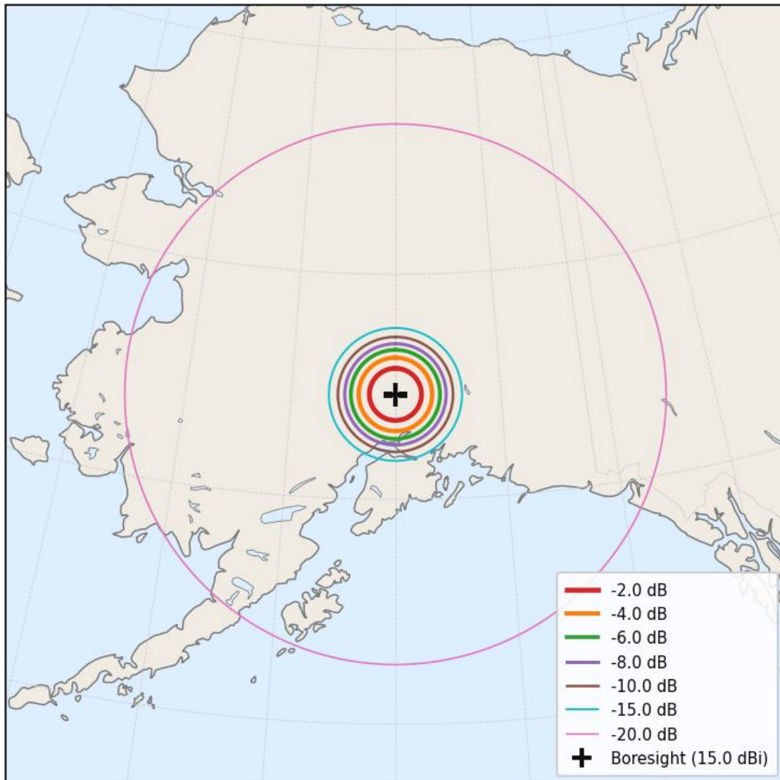
Figure 201. XTX Antenna Beam Projection over Talkeetna from Orbit altitude of 350 km
