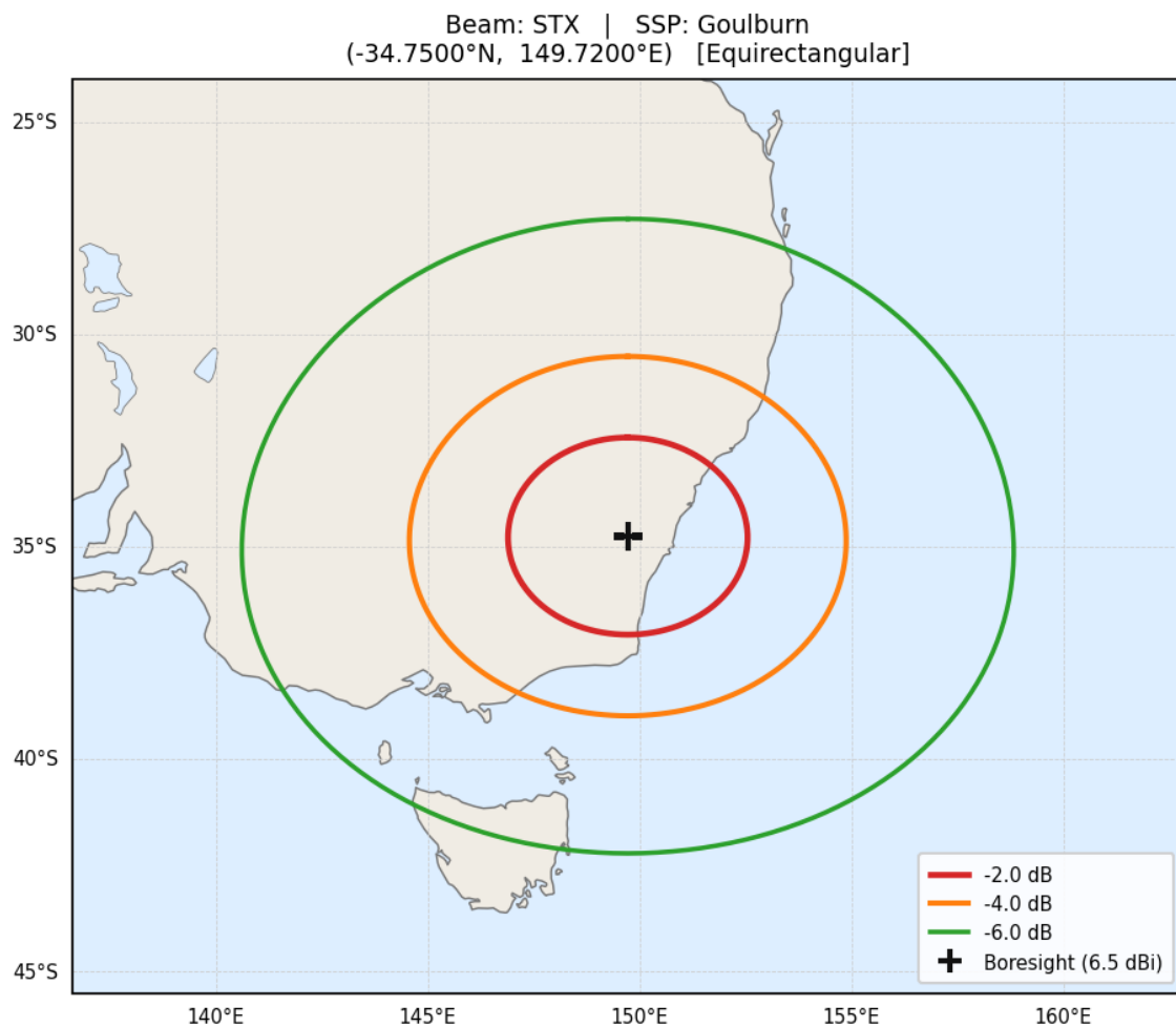
Figure 121. STX Antenna Beam Projection over Goulburn from Orbit altitude of 350 km
