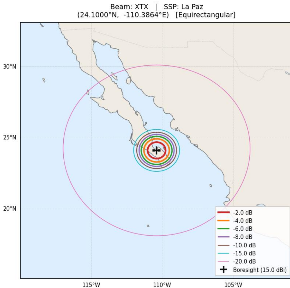
Figure 195. XTX Antenna Beam Projection over La Paz from Orbit altitude of 350 km
