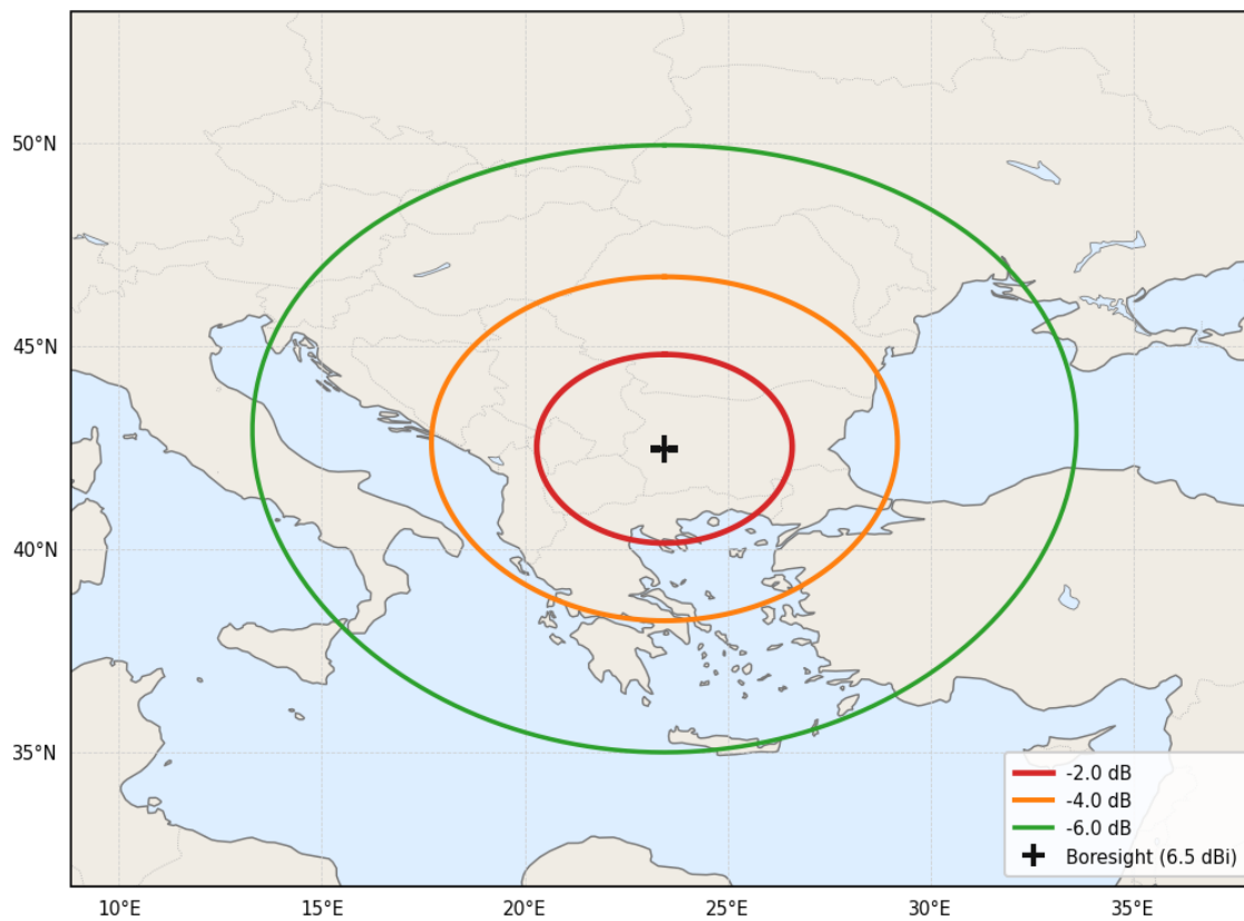
Figure 139. STX Antenna Beam Projection over Plana from Orbit altitude of 350 km
