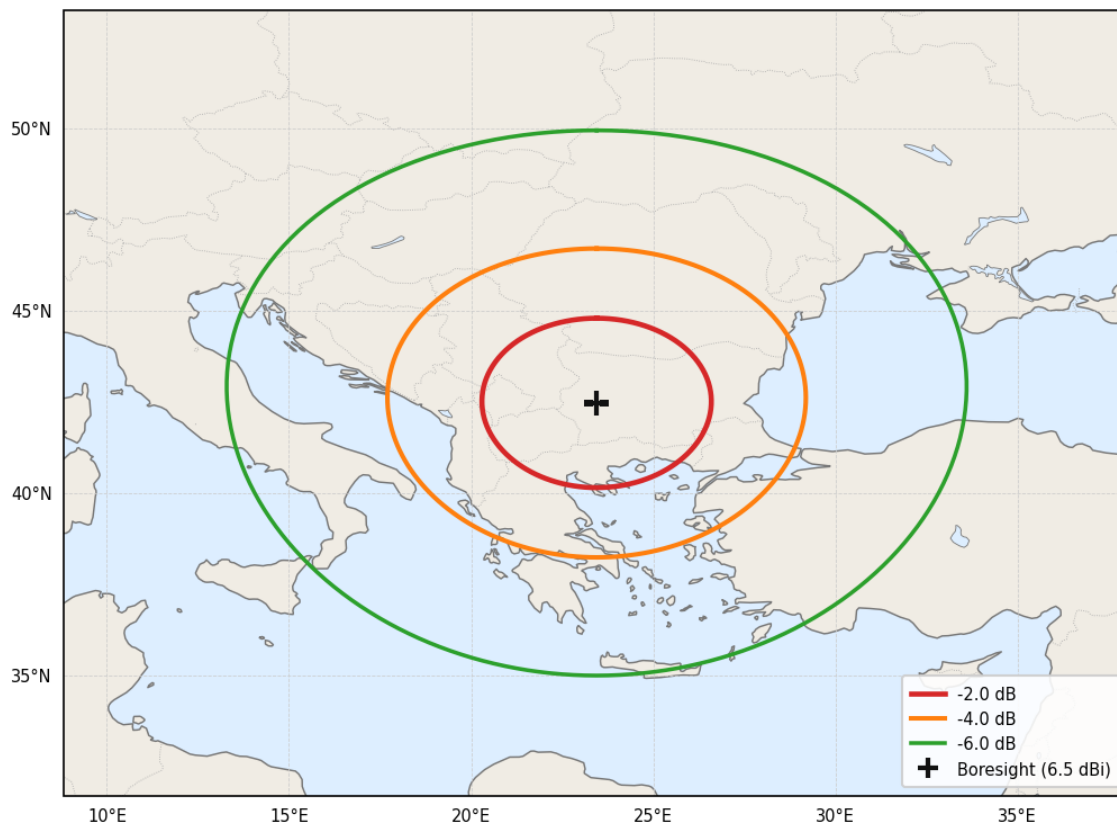
Figure 69. SRX Antenna Beam Projection over Plana from Orbit altitude of 350 km
