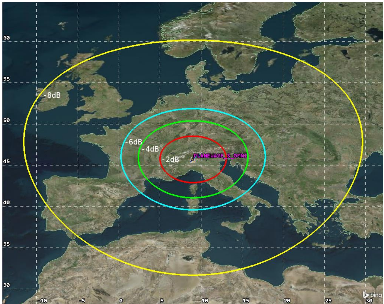
Figure 4: Dwn1 – Low Rate Omni S-band Downlink
