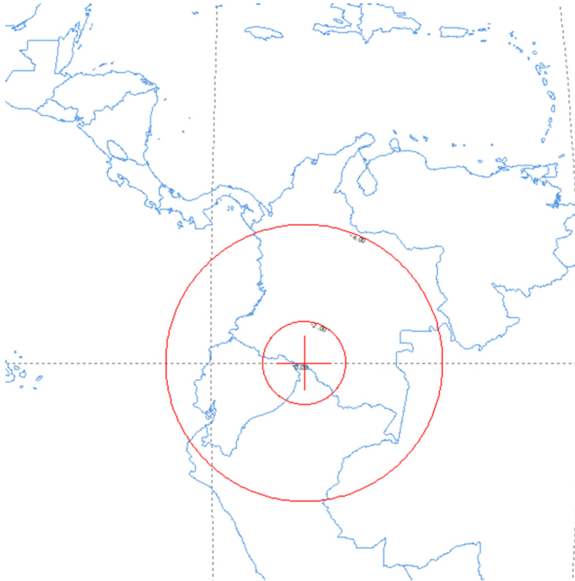
Figure 2.2-3 S-band Earth-space Antenna Beam Projection
