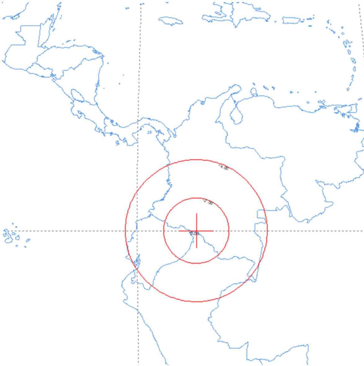
Figure 2.2-4 X-band space-Earth Antenna Beam Projection
