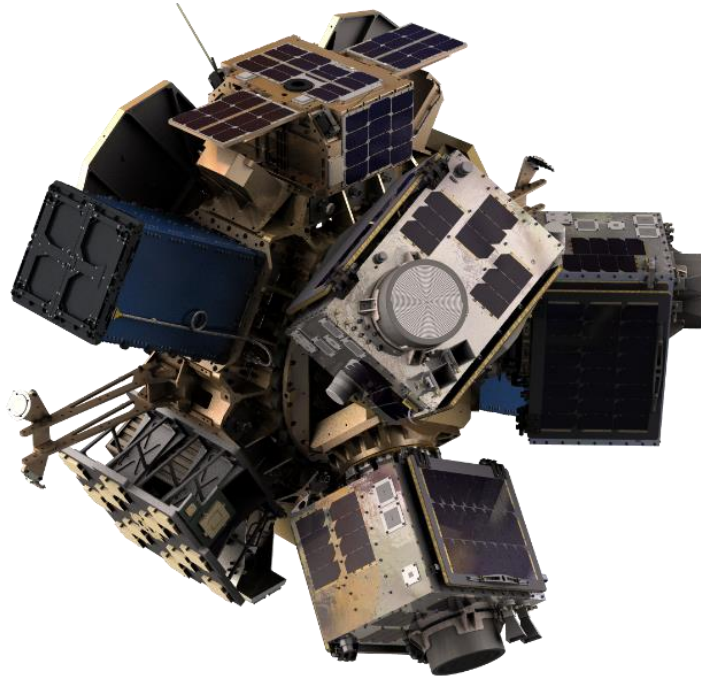
Figure 1: Physical architecture of Spaceflight’s Sherpa-AC1 with customers on a SpaceX Falcon 9 rideshare mission.
