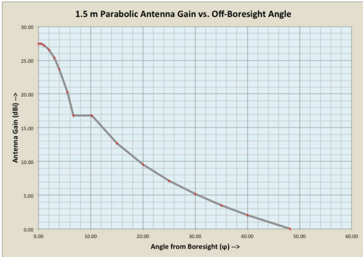
Figure C-S-TX-GS-3: Antenna Gain Profile vs. Angle from Boresight - (1.5 m Parabolic Dish Antenna)
