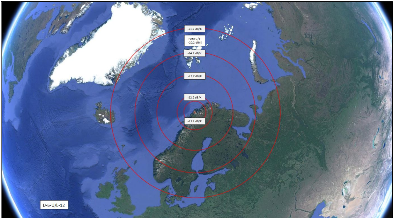
Beam Contour D-S-U/L-12: GH0St, S-band Transmit Beam; Tromsø, Norway - Figure of Merit (G/T) (dB/K)
