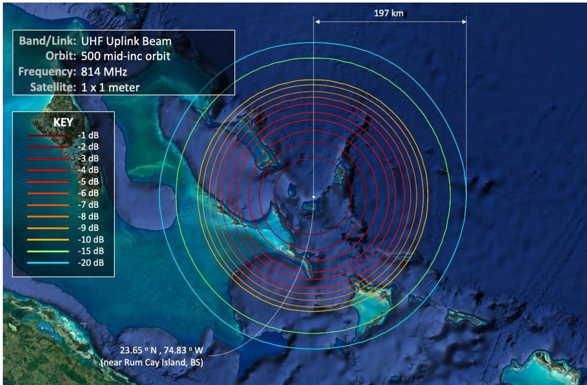
The following four (4) beam contours for the UHF-band downlink and uplink beams are relevant to the 1.5 by 1.5 meter satellite design:
