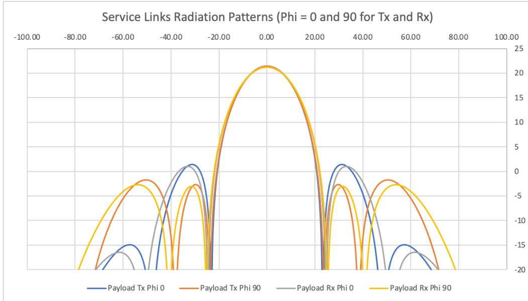
The following radiation pattern is plotted for the 24 dBiC gain antenna for azimuth angles (phi) of zero (0) and ninety (90) degrees relative to boresight, and the pattern demonstrates a 25 dB Chebyshev amplitude taper for peak side lobes just below zero. The amplitude taper on the array may be reconfigured and is dynamic.
