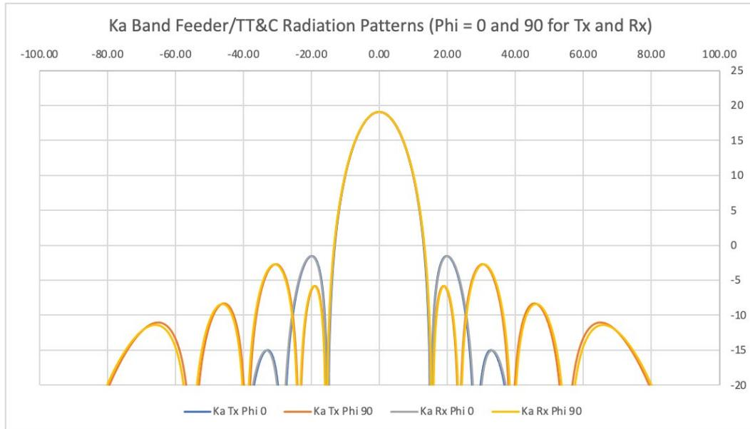
The following radiation pattern is plotted for the 23 dBiC gain antenna for azimuth angles (phi) of zero (0) and ninety (90) degrees relative to boresight, and the pattern demonstrates a 23 dB Chebyshev amplitude taper for peak side lobes just below zero.
