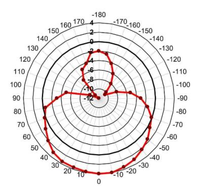
The S-band patch antenna beam contour on the ground is illustrated below. At the -4 dB point the contour is over the horizon so only the -2 dB contour and the horizon contours are shown.
