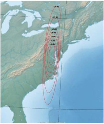
The figure below shows the S-Band Patch Antenna beampattern.
