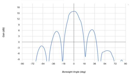
The figure below shows the X-band Patch Antenna beampattern.
