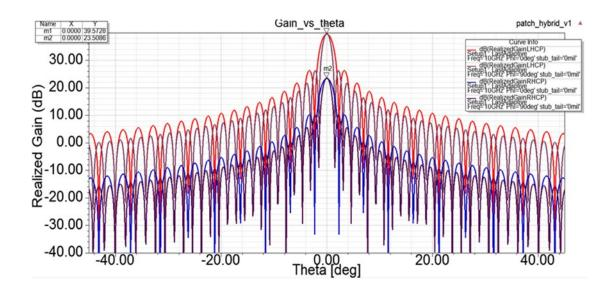
The SAR transmit beam pattern (short side) is shown in the figure below.
