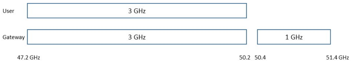
Figure III-8. Uplink Communications Frequency Plan
