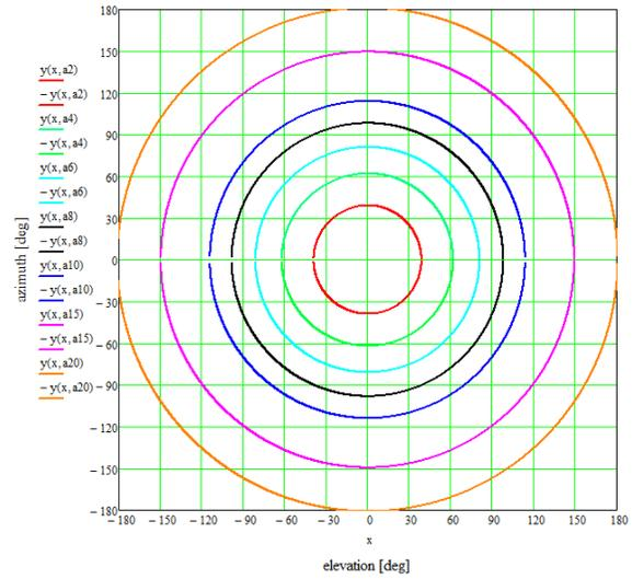
**Figure A.3.2-2: VLEO Beacon Beam Gain Contours**
