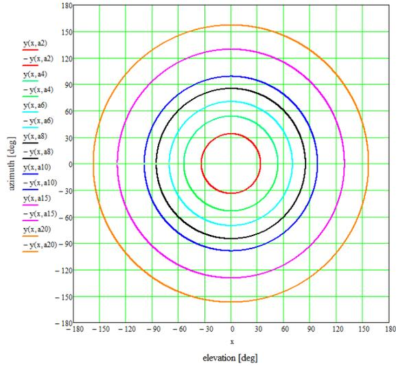
**Figure A.3.2-1: LEO Beacon Beam Gain Contours**
