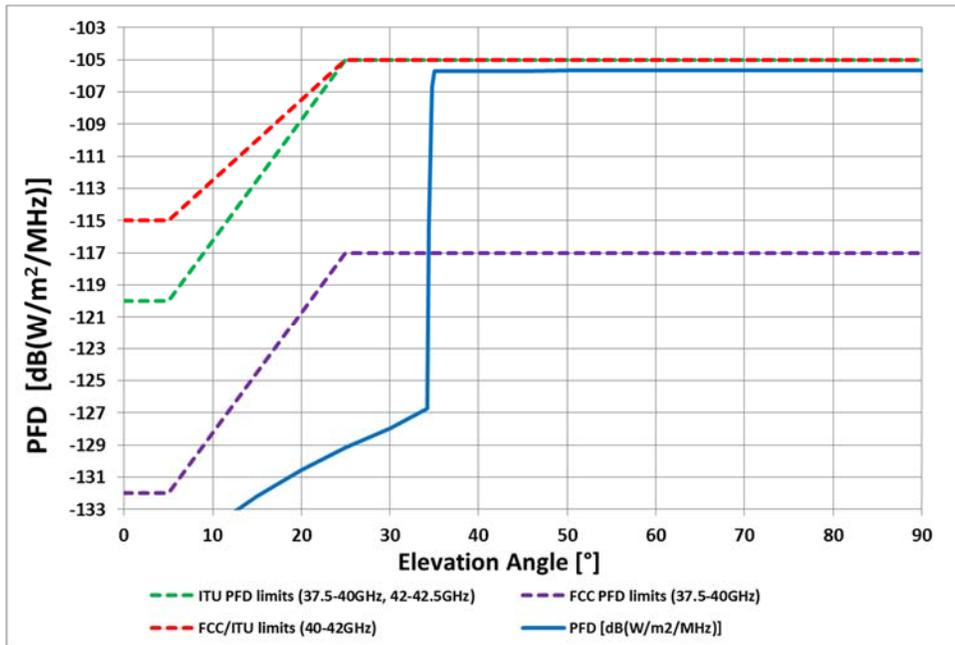
**Figure A.7-2: VLEO Constellation Downlink PFD Levels in the 37.5-42.5 GHz Band**
