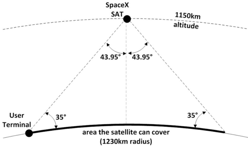
**Figure A.3.1-1: Steerable Service Range of LEO Beams (1,150 km)**
