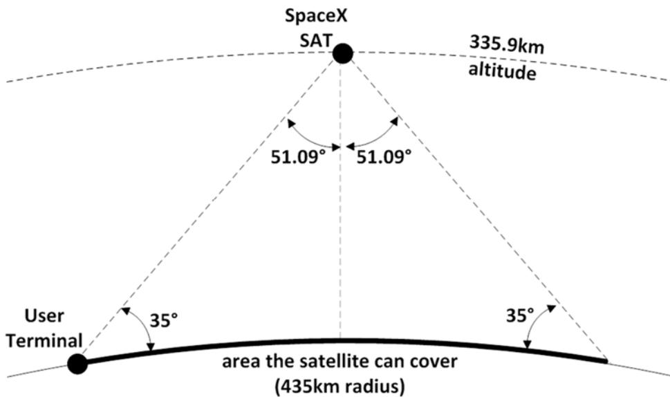
**Figure A.3.1-2: Steerable Service Range of VLEO Beams (335.9 km)**
