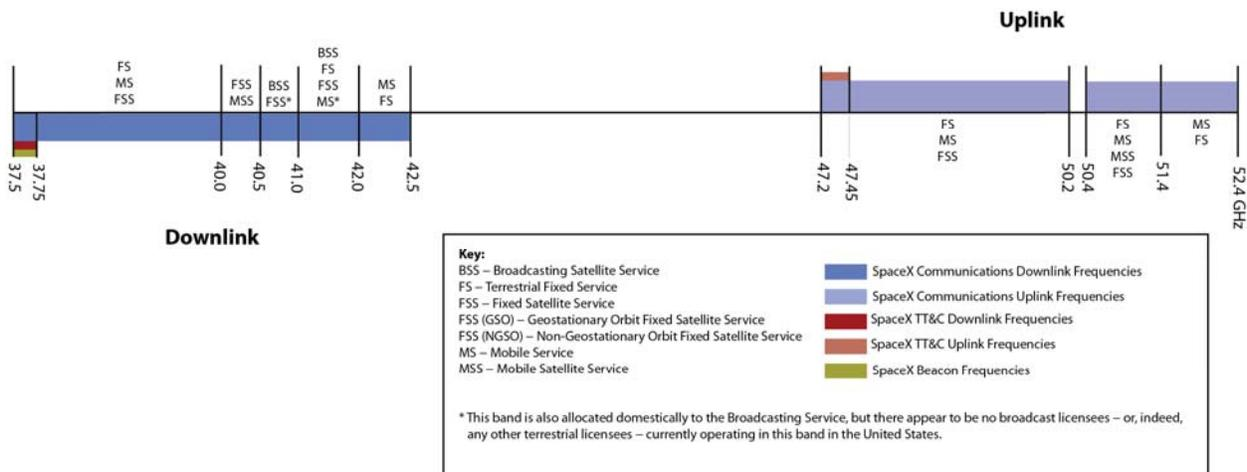
**Figure A.2-4: V-Band Spectrum Used by the SpaceX System**
