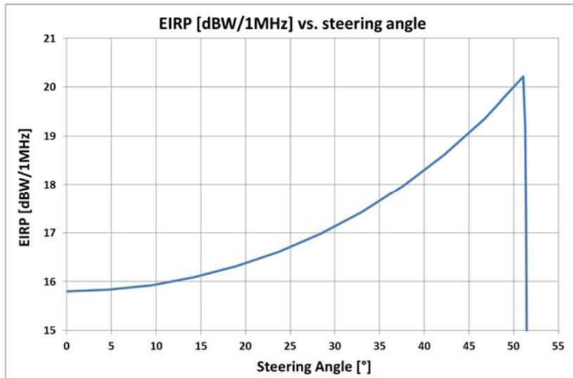
Figure A.3.1-8: VLEO EIRP Density Variation by Beam Steering Angle
