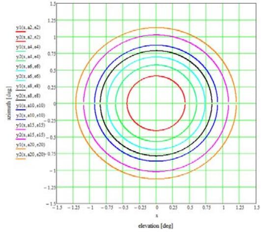
**Figure A.3.1-5: Beam Contours at 40 Degrees Elevation**
