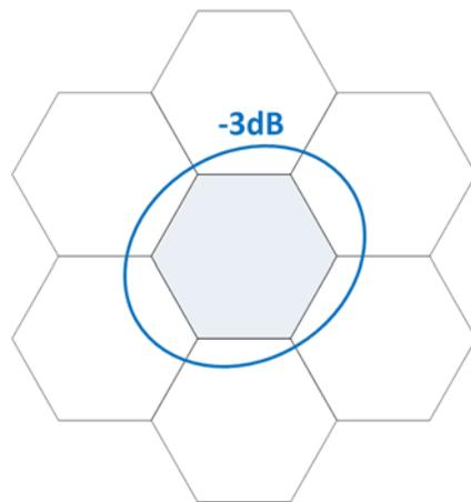
**Figure A.3.1-6: Intended Beam Coverage Area**
