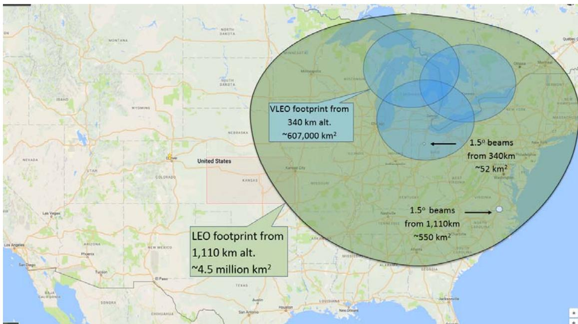
**Figure A.2-1: Comparative Illustration of LEO and VLEO Coverage**
