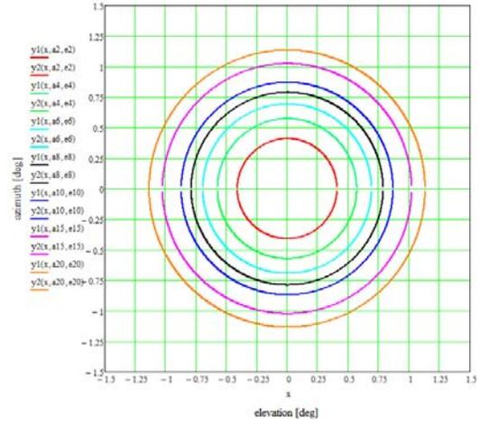
**Figure A.3.1-4: Beam Contours at 20 Degrees Elevation**
