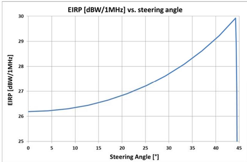
Figure A.3.1-7: LEO EIRP Density Variation by Beam Steering Angle
