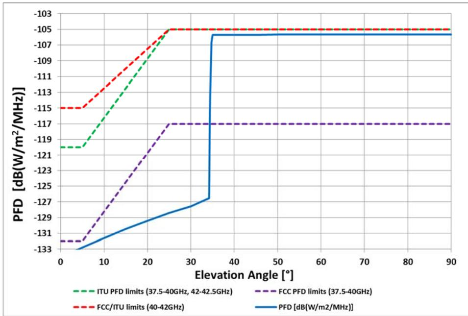
**Figure A.7-1: LEO Constellation Downlink PFD Levels in the 37.5-42.5 GHz Band**
