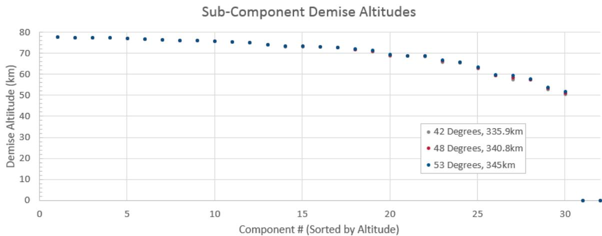
Several objects were identified as components of interest. This reflected objects which had a distinct mass, quantity, or shape factor which made them of particular concern during re-entry analysis. Those components and their corresponding demise altitudes are provided in the tables below:
