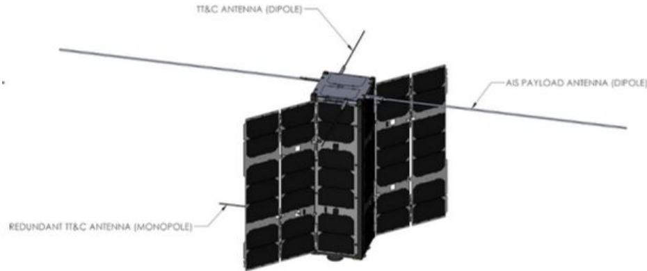
Figure 1. LEMUR-2 in Fully Deployed Configuration
