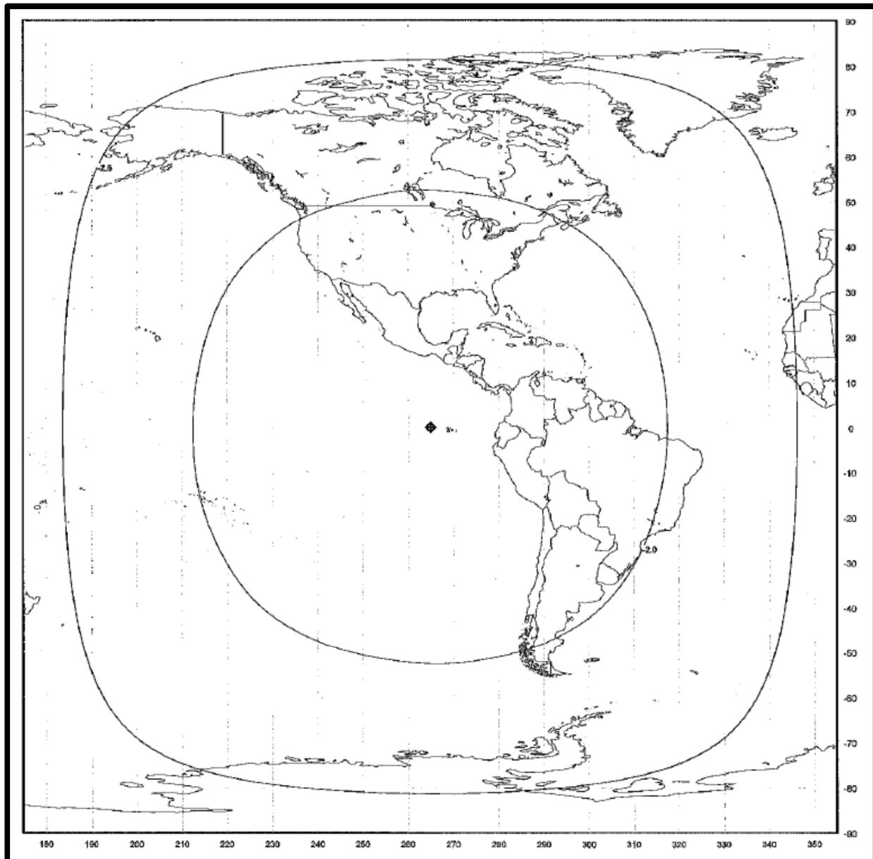
**EXHIBIT 5B-5: TELEMETRY TRANSMIT BEAM (back-up)**
