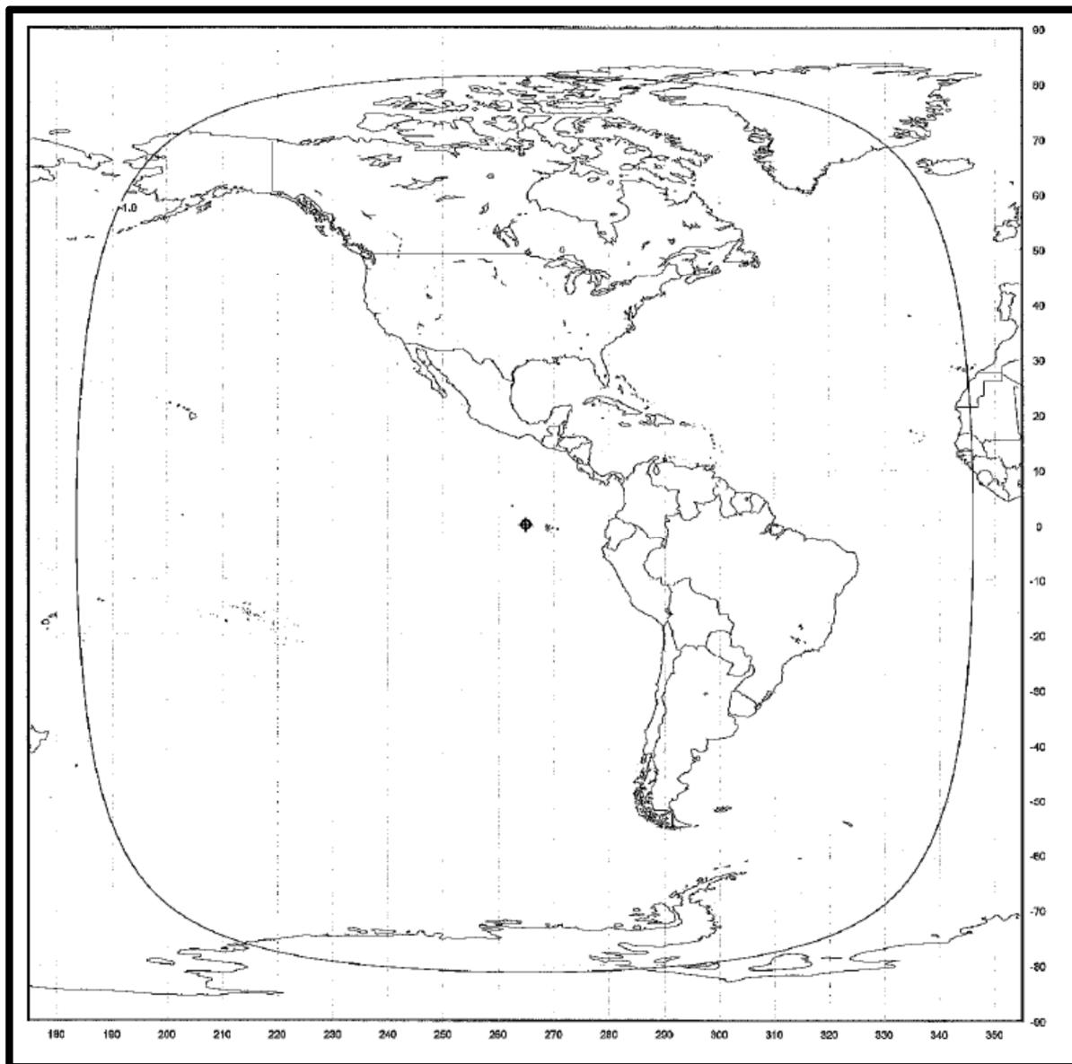
**EXHIBIT 5B-4: TELEMETRY TRANSMIT BEAM (on-station)**
