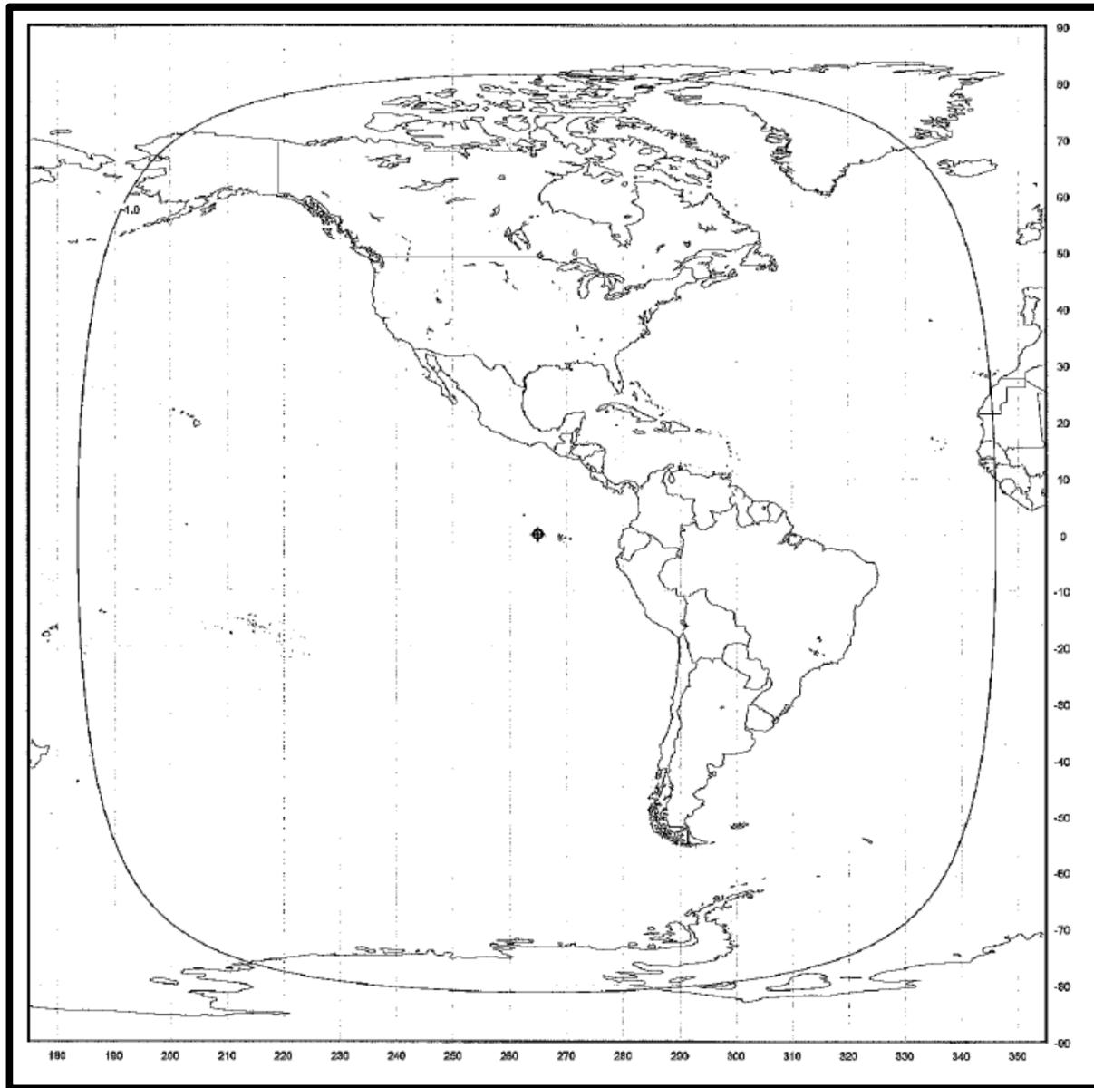
**EXHIBIT 5B-6: TELEMETRY TRANSMIT BEAM (back-up)**
