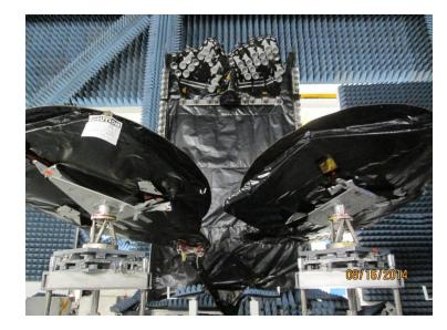
Intelsat IS 29e satellite elements, built by Boeing Antenna in test (left)
