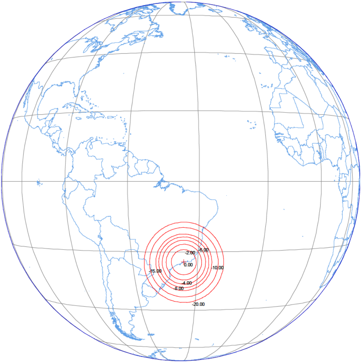
Figure B-2. DIRECTV KU-45W Receive Beam 2
