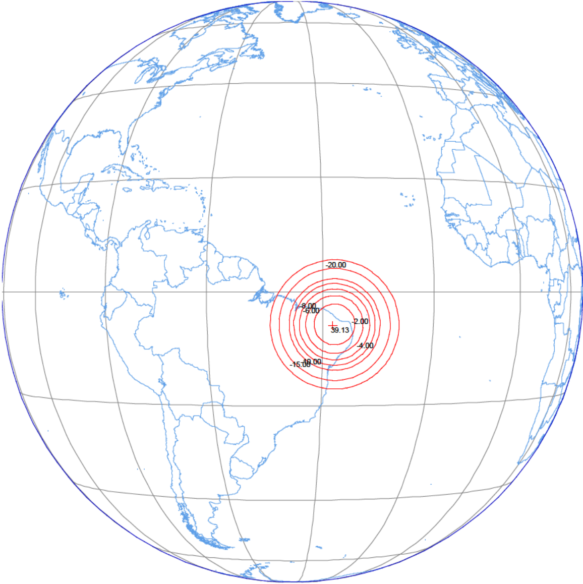
Figure B-1. DIRECTV KU-45W Receive Beam 1
