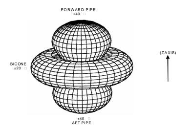
Figure B-4. DIRECTV KU-79W Wide Beam TT&C Antenna Coverage
