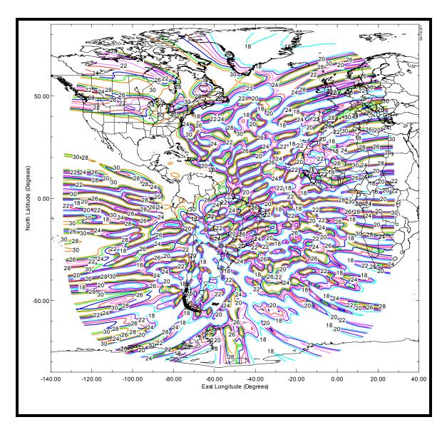
Absolute cross-polarization isolation contours shown: 30, 28, 26, 24, 22, 20, 18 dB.
