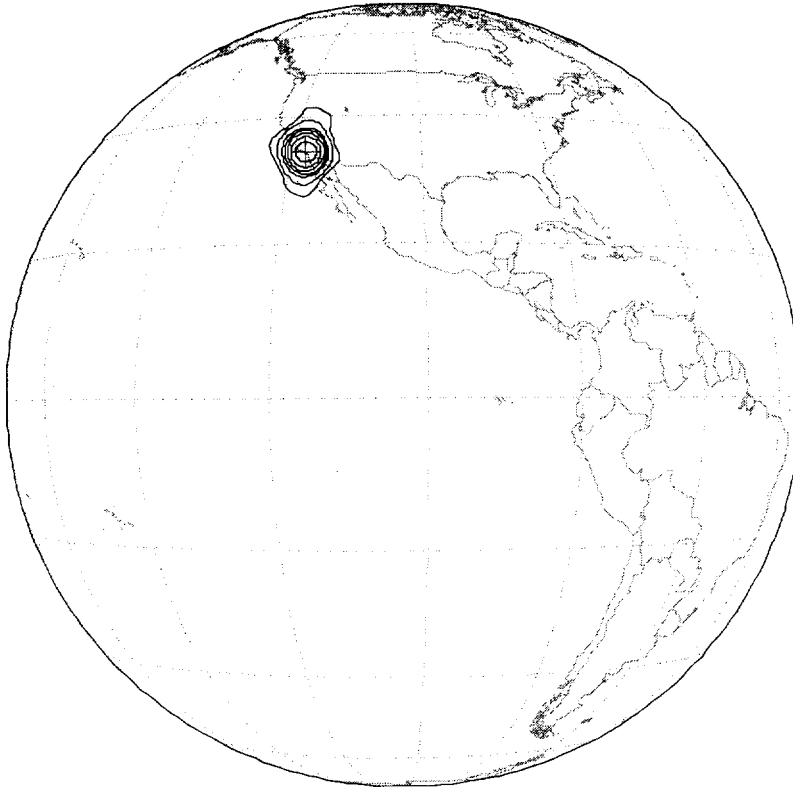
Figure C-4. DIRECTV 10 Typical Spot Beam
