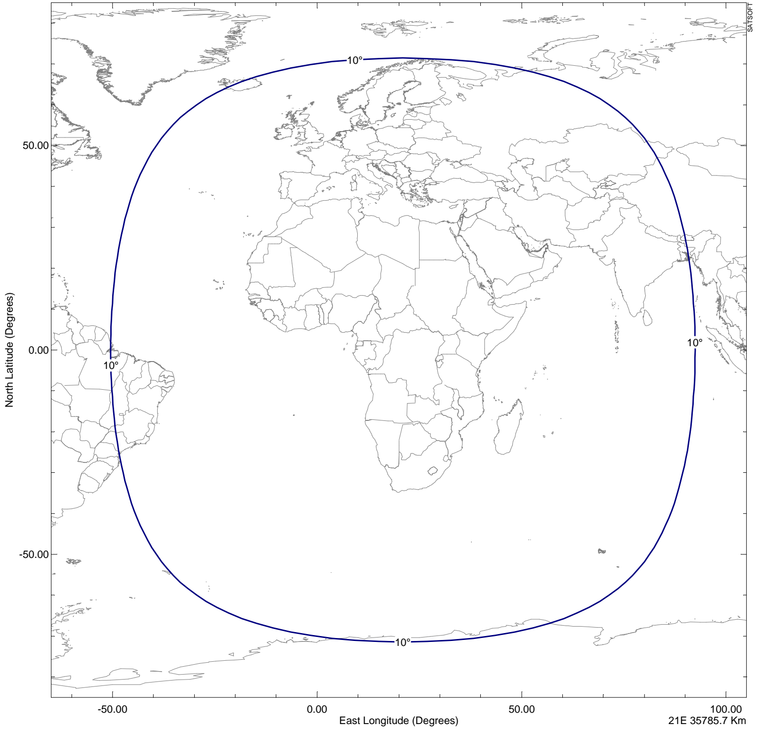
Figure 3: Telemetry Downlink Service Area (10° Elevation Contour)
