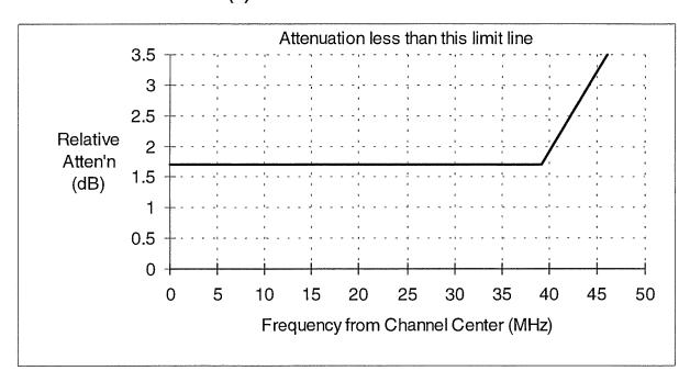
FIGURE 8 - OUT-OF-BAND TRANSPONDER FILTER RESPONSES
