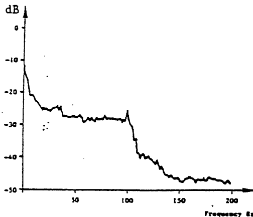
FIGURE 11 - Spectrum of signal envelope (suburban area); vehicle speed: 40 km/h frequency: 1.5 GHz [Jongeijans, 1986]
