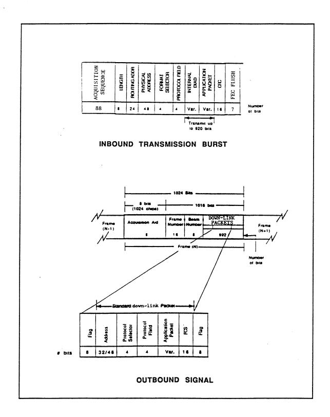
Figure 2. RDSS Signal Structure
