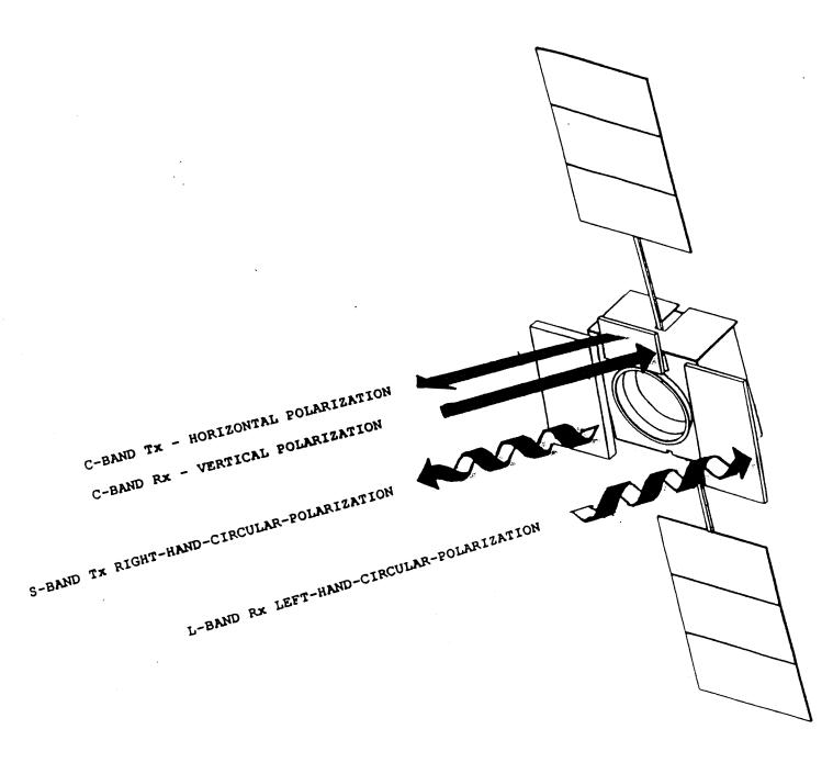
Figure 4. Geostar Single Beam Dedicated RDSS Satellite Design
