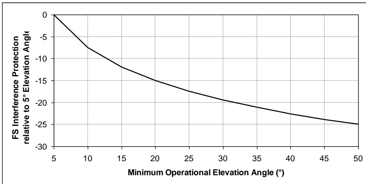
Figure 21, Interference Protection with Respect to FS Systems as a Function of the Minimum Operational Angle of Separation between the Active Pleiades Satellite and the GSO Arc
