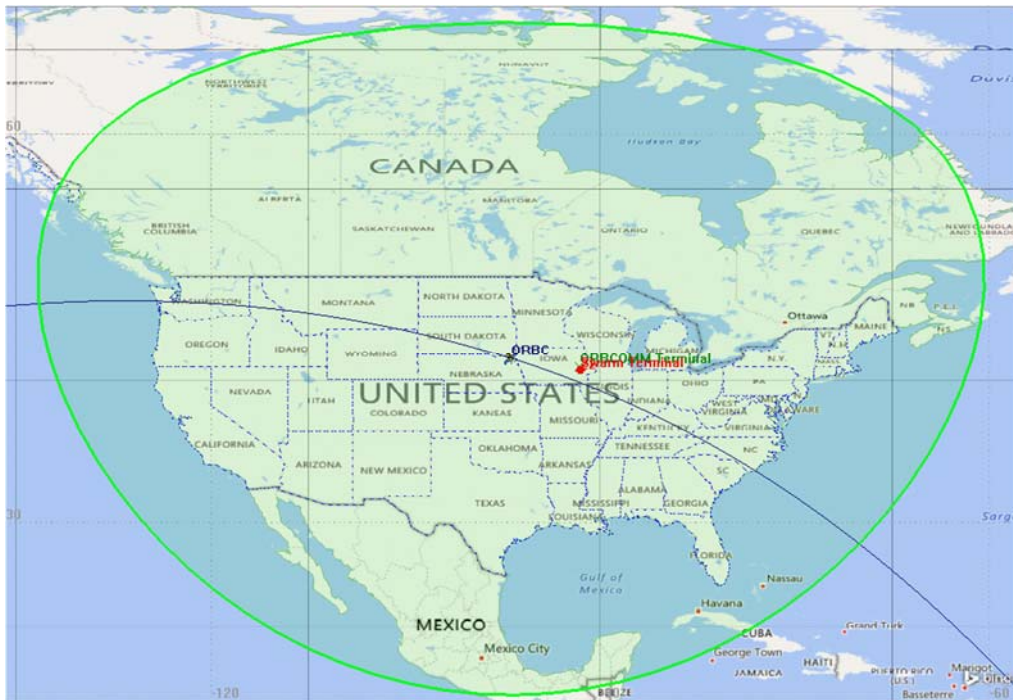
Figure 2 – ORBCOMM Coverage Area in which a Swarm Transmission would Interfere With a Co-frequency ORBCOMM Uplink Transmission
