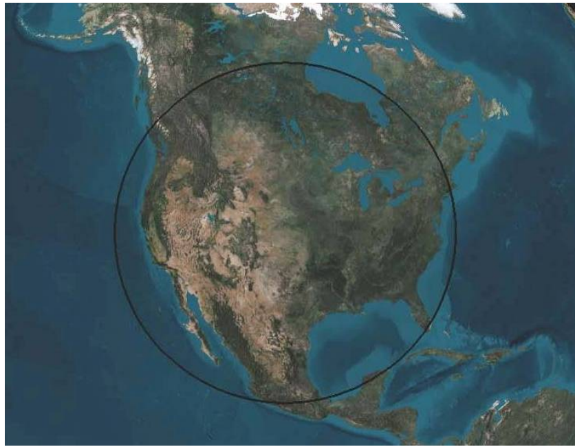
Figure 1 Representative Single OG2 Satellite Footprint Altitude = 715 km, User Minimum Elevation Angle Mask = 5°
