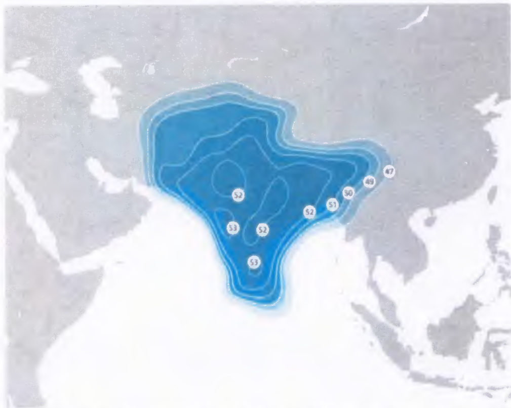
Figure 1. Downlink EIRP contours of the NSS-12 satellite in the band 12.25-12.50 GHz.
