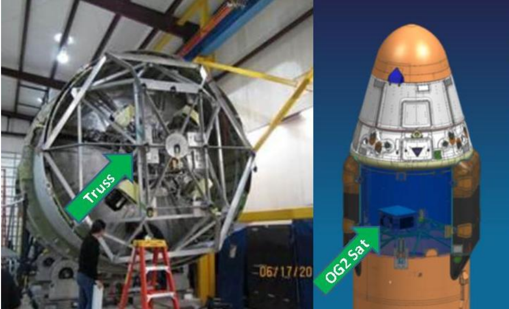
Figure 1: OG2 interface truss structure mated to Falcon 9 second stage extension
