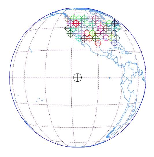
ATCONTACT 115W Beam Array and Coverage Pattern
