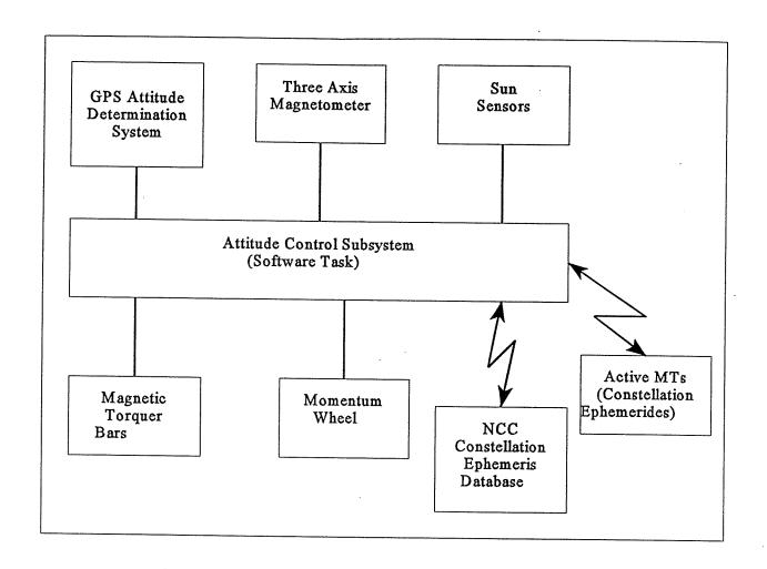
The sun sensor will be located on a deployed solar array panel on one side of the satellite, as close as practical to the panel axis <u>center</u>line. Backup sensors will be a single three (3) axis magnetometer and a redundant sun sensor located on the deployed solar array panel on the opposite side of the satellite.
