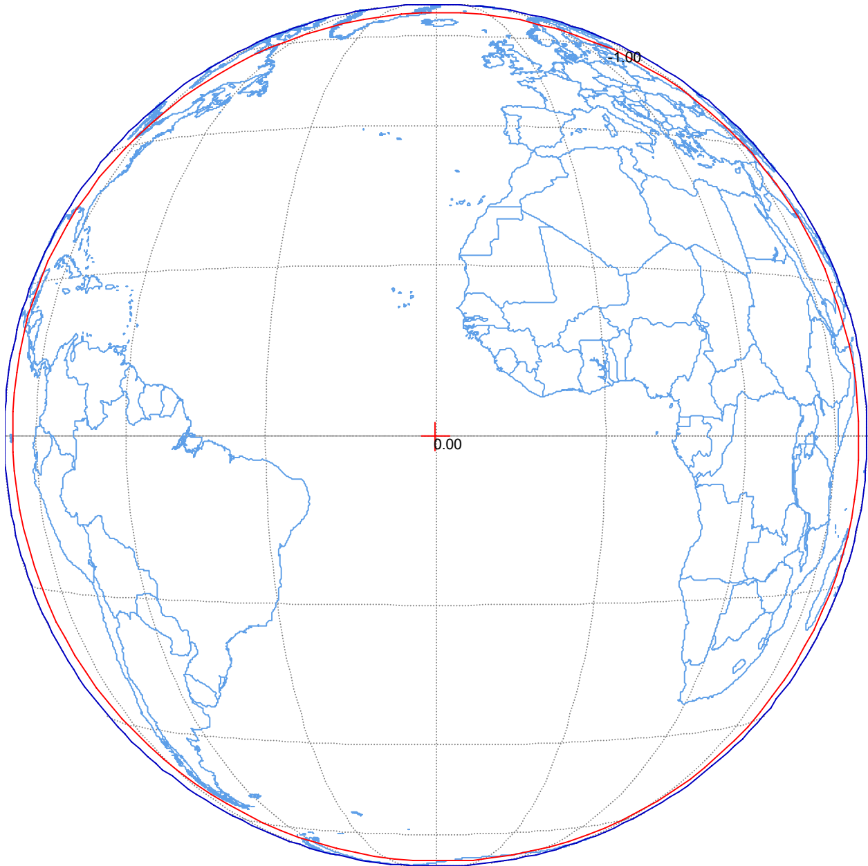
Figure B-24. Telemetry Carrier Earth Facing Transmit Horn 10 Maximum EIRP = 10 dBW; Maximum transmit gain = 11.3 dBi Polarization RHCP Schedule S beam designator: TLM
