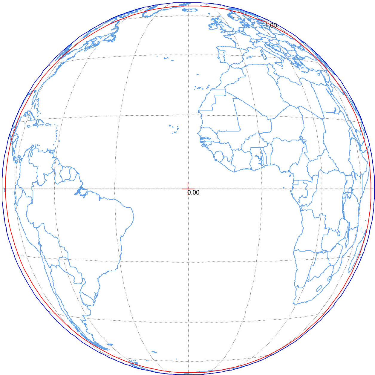
Figure B-25. C-band Tracking Beacon Earth Facing Transmit Horn 11 Maximum EIRP = 11 dBW Maximum transmit gain = 11.3 dBi Polarization Vertical Linear Schedule S beam designator: BNC
