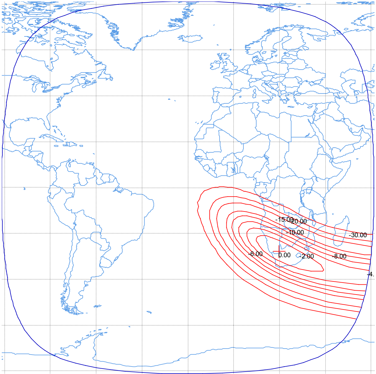
Figure B-19. Spot 2 Uplink Beam Peak G/T = 9.1 dB/K Peak Beam Gain = 37.6 dBi Min. Saturation Flux Density = -99 dBW/m 2 Polarization Vertical or Horizontal Linear Schedule S beam designators: S2AU and S2BU
