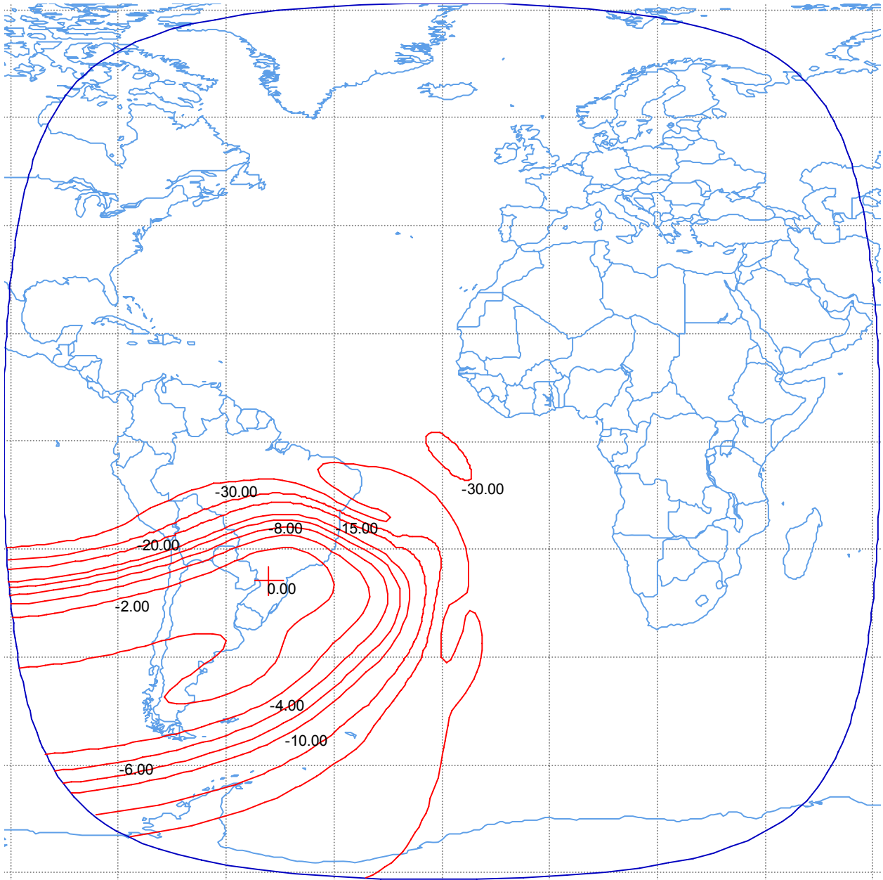
Figure B-11. South West Zone Uplink Beam Peak G/T = 1.5 dB/K Peak Beam Gain = 30.8 dBi Min. Saturation Flux Density = -96 dBW/m 2 Polarization RHCP Schedule S beam designator: SWZU
