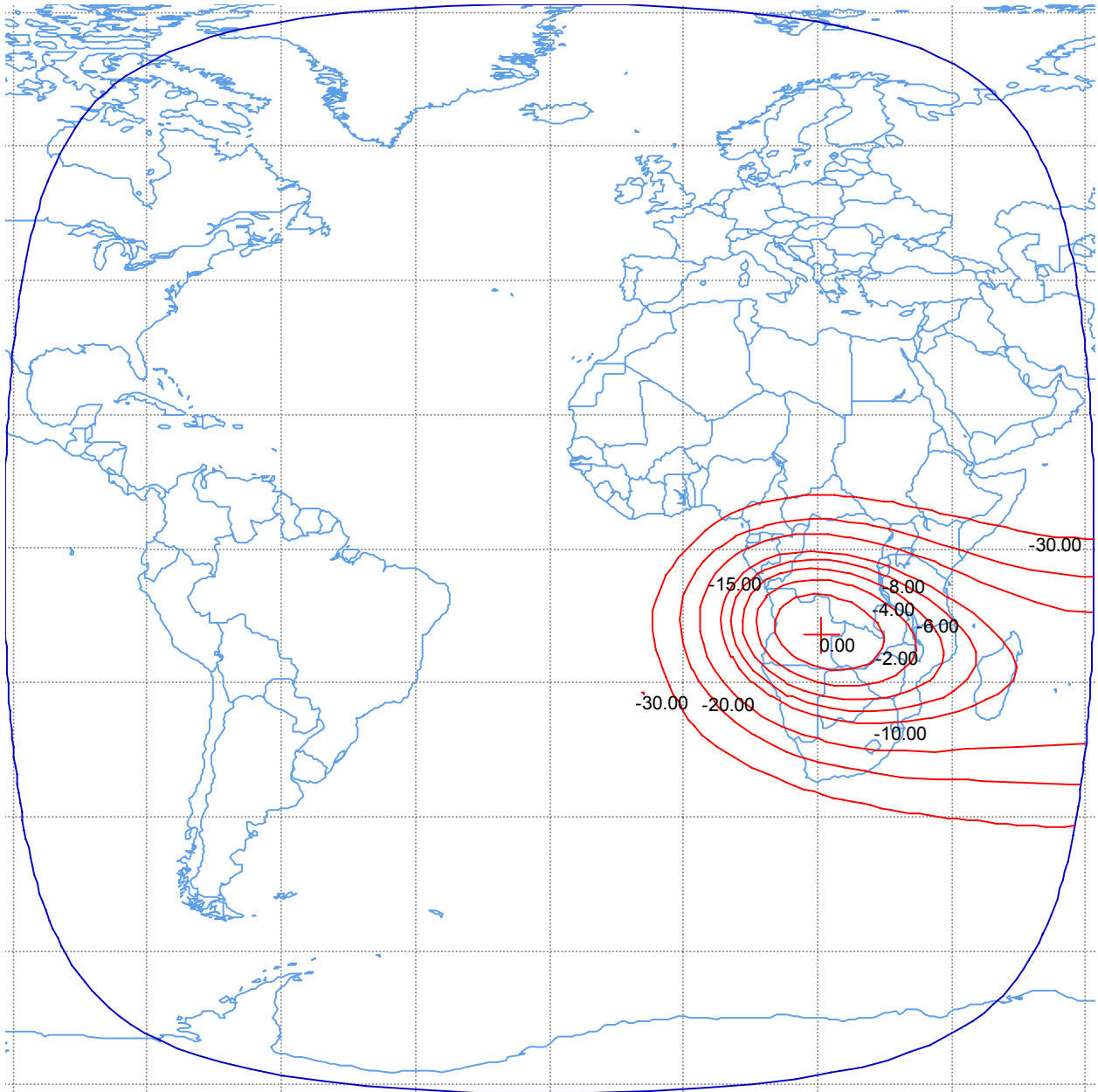
Figure B-27. Ku-band Tracking Beacon with Spot 1 antenna Maximum EIRP = 9 dBW Maximum transmit gain = 37.9 dBi Polarization Linear Vertical or Horizontal Schedule S beam designator: BNK2
