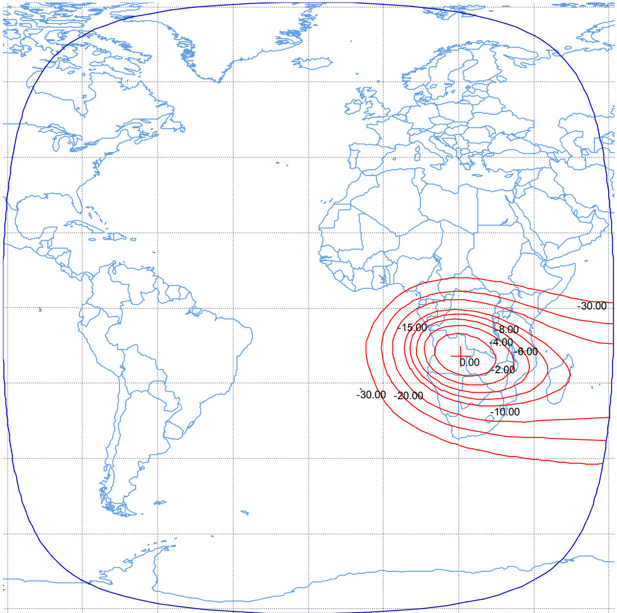
Figure B-18. Spot 1 Downlink Beam Peak EIRP = 52.1 dBW Peak Beam Gain = 37.9 dBi Polarization Vertical or Horizontal Linear Schedule S beam designators: S1AD and S1BD
