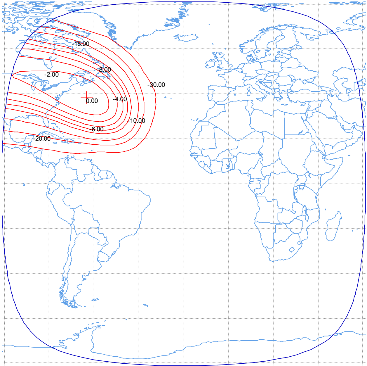
Figure B-8. North West Zone Downlink Beam Peak EIRP = 42.7 dBW Peak Beam Gain = 35.0 dBi Polarization LHCP Schedule S beam designator: NWZD
