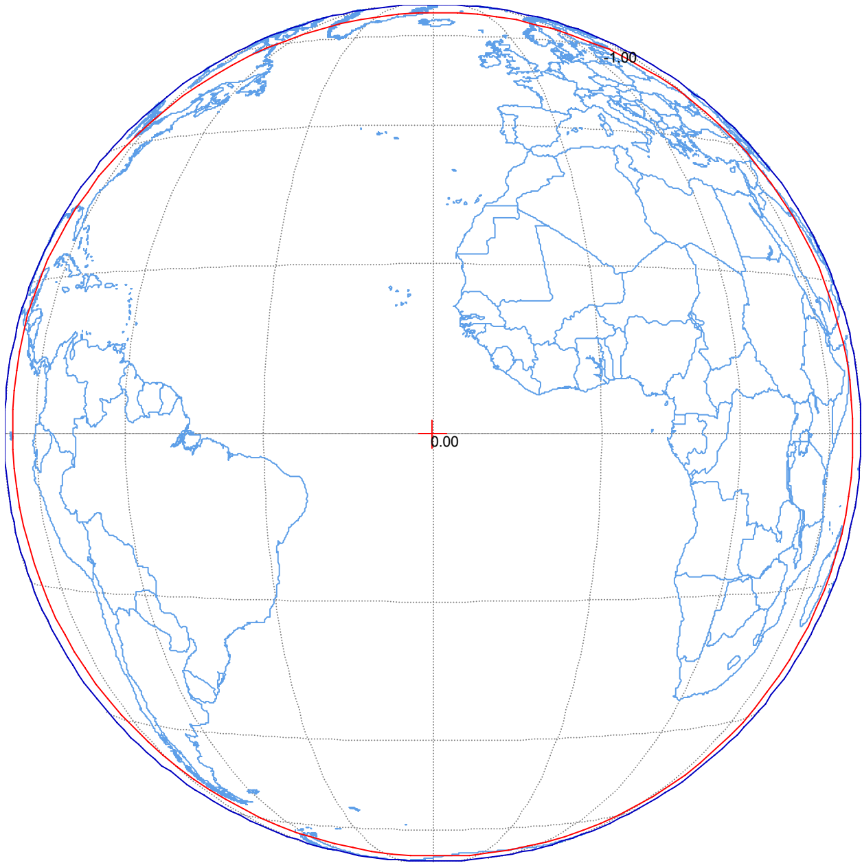
Figure B-26. Ku-band Tracking Beacon Earth Facing Transmit Horn 12 Maximum EIRP = 13 dBW Maximum transmit gain = 20.3 dBi Polarization RHCP Schedule S beam designator: BNK1
