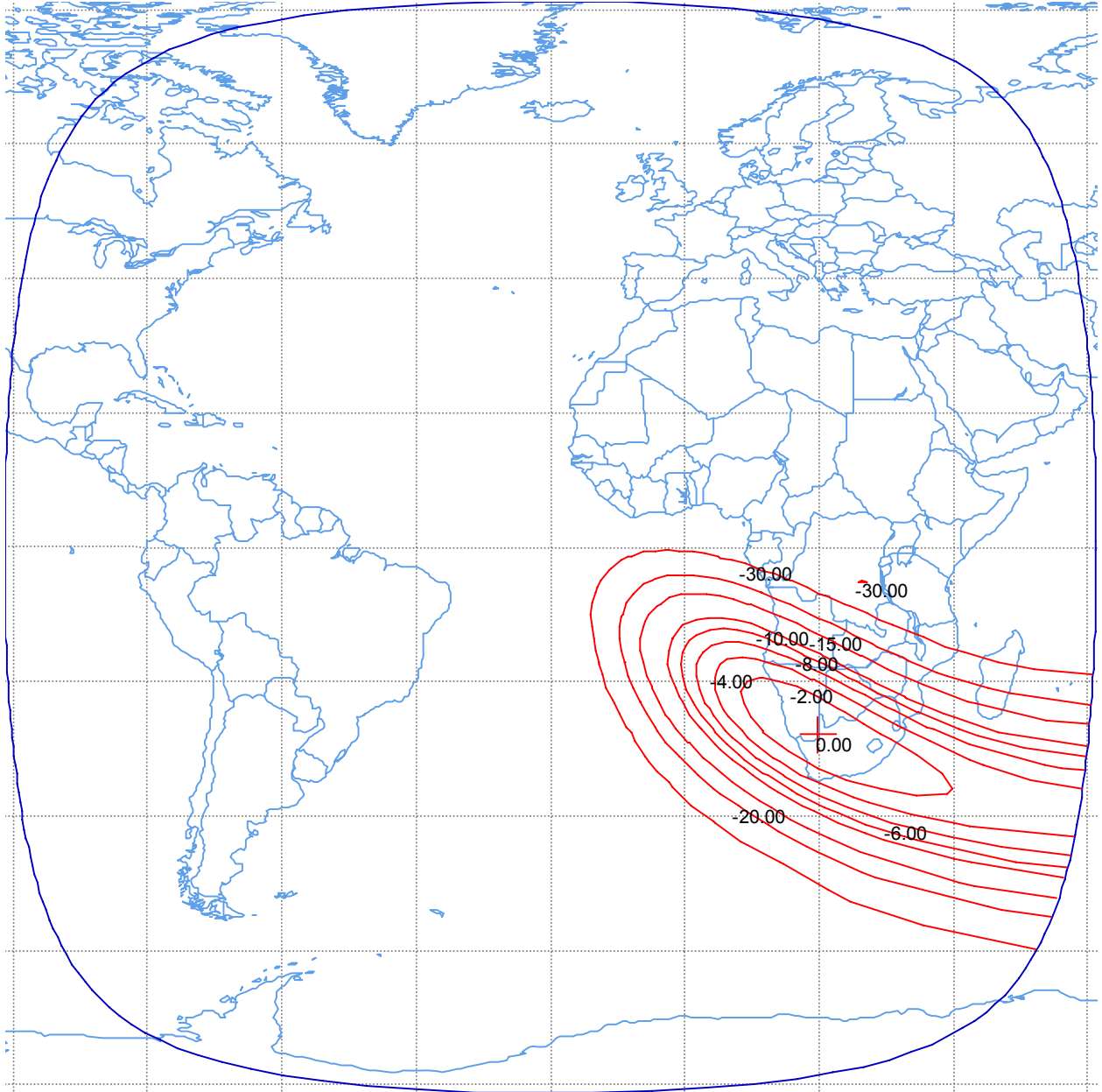
Figure B-20. Spot 2 Downlink Beam Peak EIRP = 51.3 dBW Peak Beam Gain = 36.9 dBi Polarization Vertical or Horizontal Linear Schedule S beam designators: S2AD and S2BD
