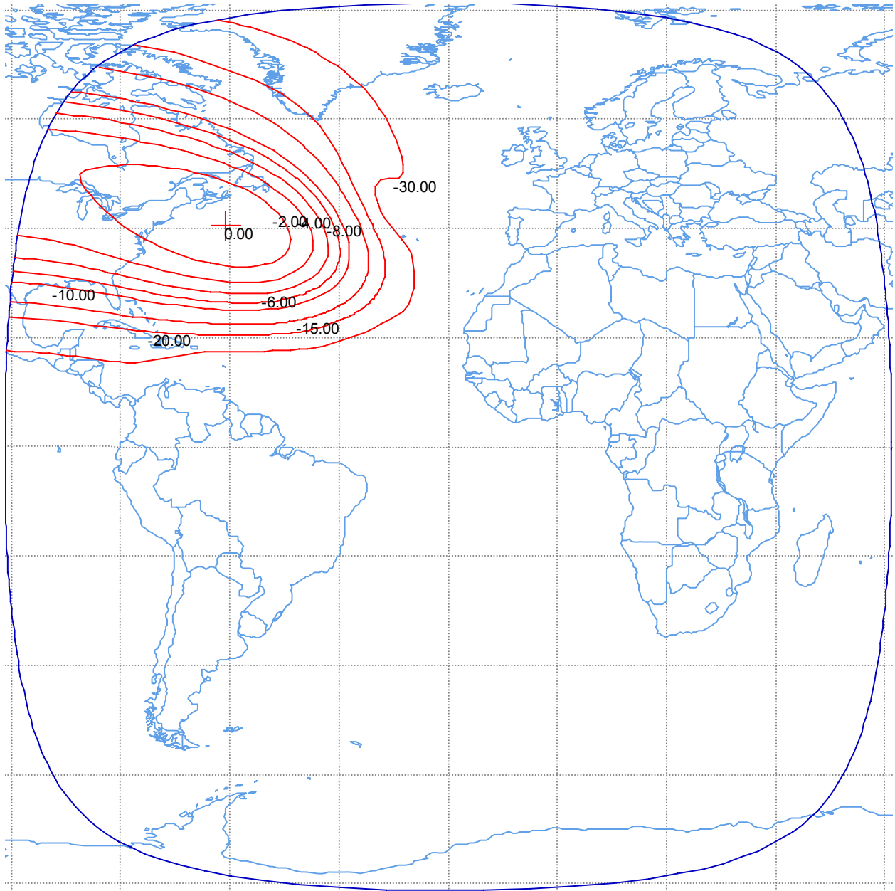
Figure B-7. North West Zone Uplink Beam Peak G/T = 4.8 dB/K Peak Beam Gain = 34.3 dBi Min. Saturation Flux Density = -99 dBW/m 2 Polarization RHCP Schedule S beam designator: NWZU
