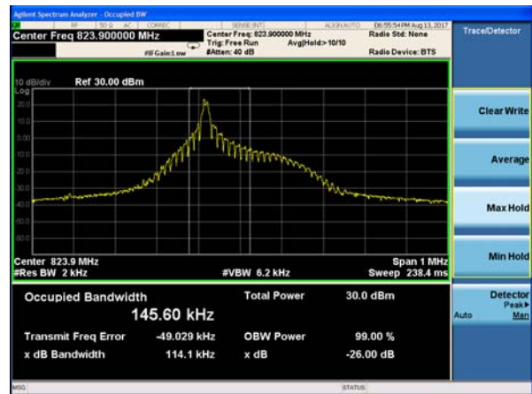
NB-IOT Band 26 BPSK 15kHz 1@0 CH-High
