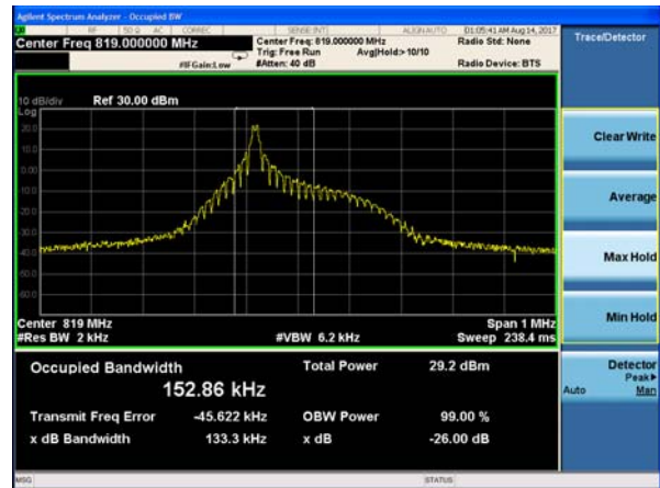
NB-IOT Band 26 BPSK 15kHz 1@0 CH-High
