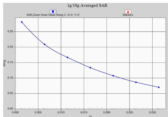
Fig. 1-15 Z-Scan at power reference point (LTE B5 Head)
