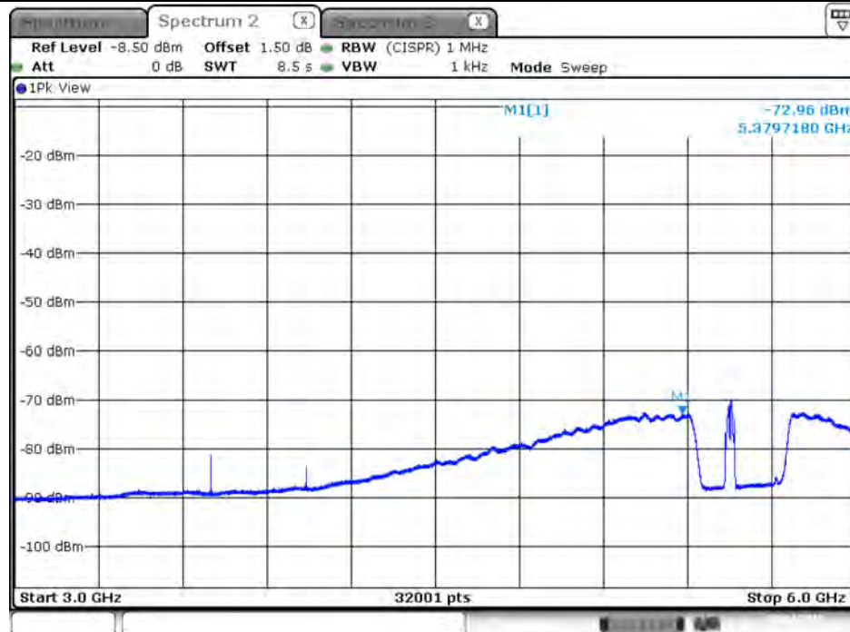
Plot on Configuration VHT40 / 5550 MHz / Average / Port 4 / 3GHz~6GHz
