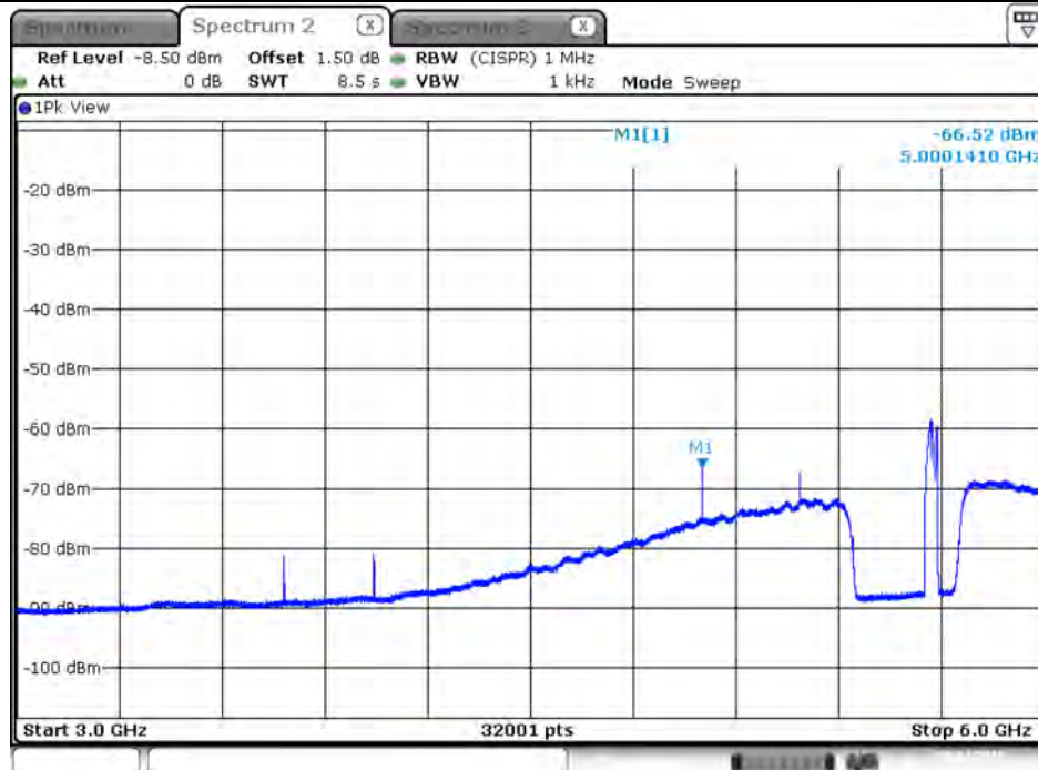
Plot on Configuration VHT40 / 5670 MHz / Average / Port 2 / 3GHz~6GHz
