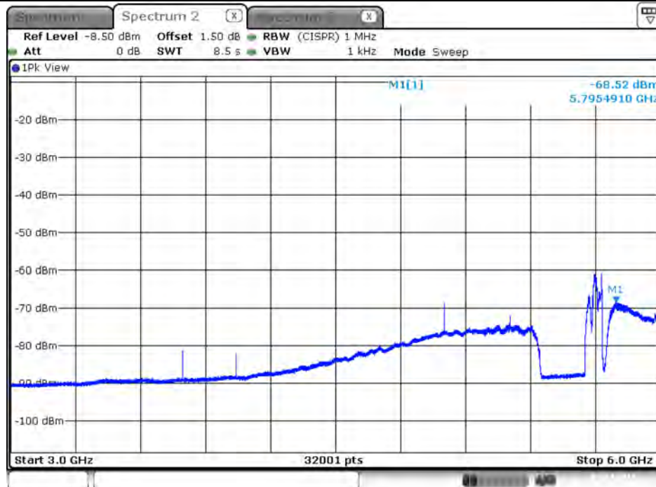
Plot on Configuration VHT80 / 5690 MHz / Average / Port 2 / 3GHz~6GHz
