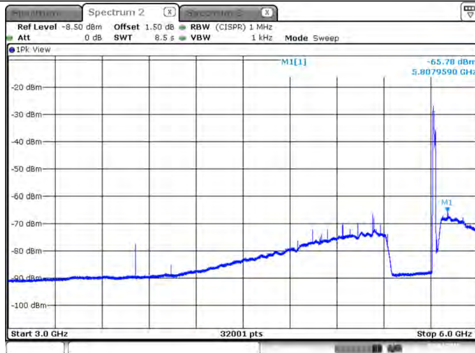
Plot on Configuration VHT20 / 5720 MHz / Average / Port 1 / 3GHz~6GHz
