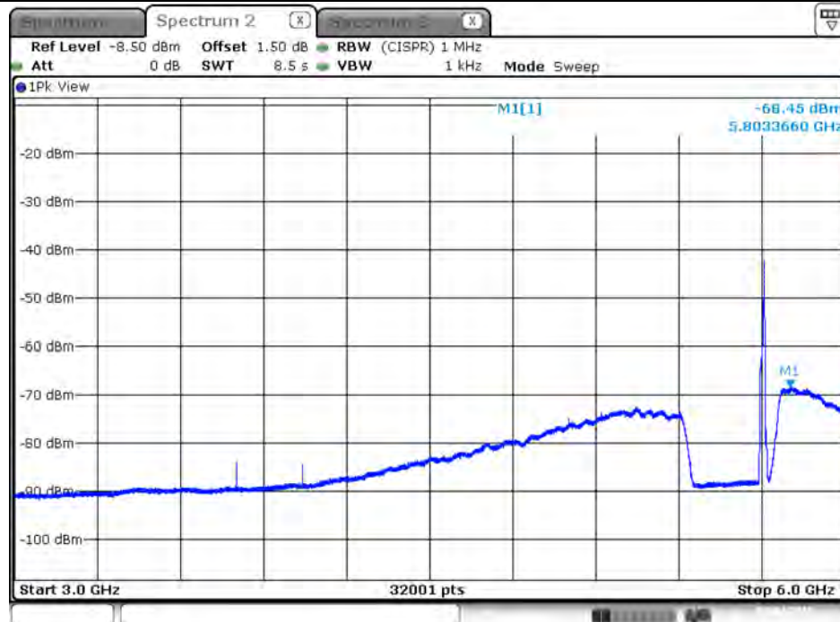
Plot on Configuration VHT20 / 5700 MHz / Average / Port 4 / 3GHz~6GHz
