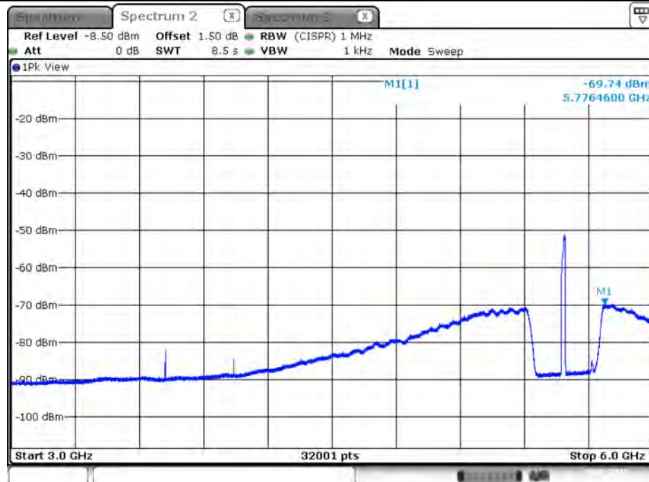
Plot on Configuration VHT20 / 5580 MHz / Average / Port 4 / 3GHz~6GHz
