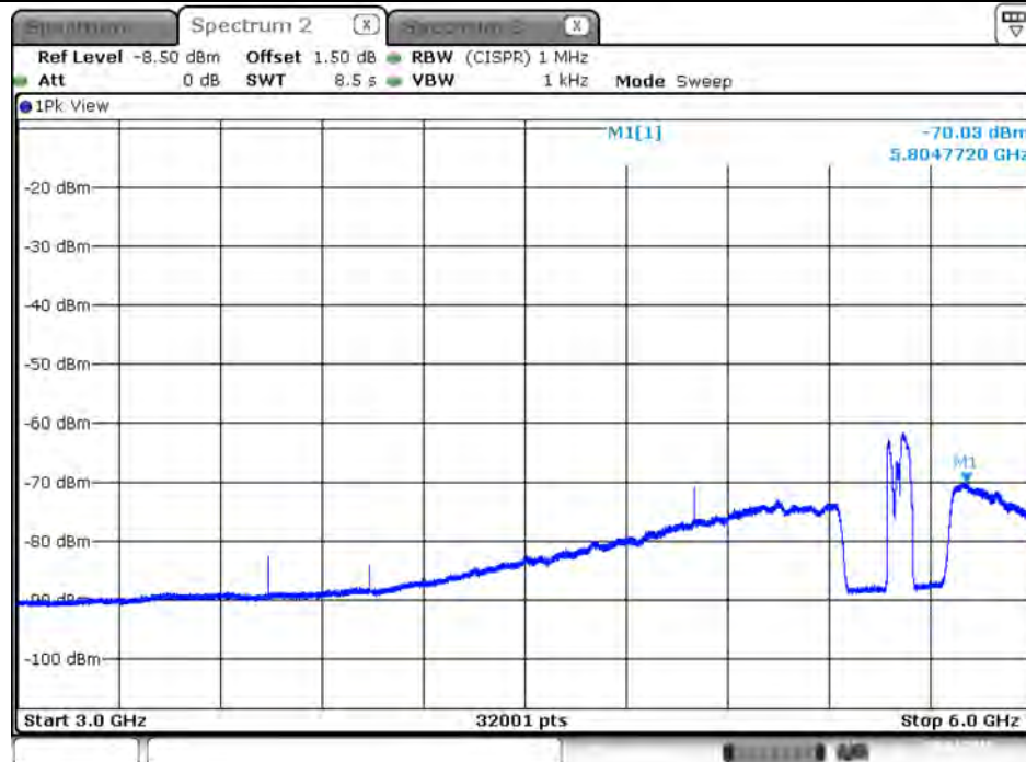
Plot on Configuration VHT80 / 5610 MHz / Average / Port 4 / 3GHz~6GHz
