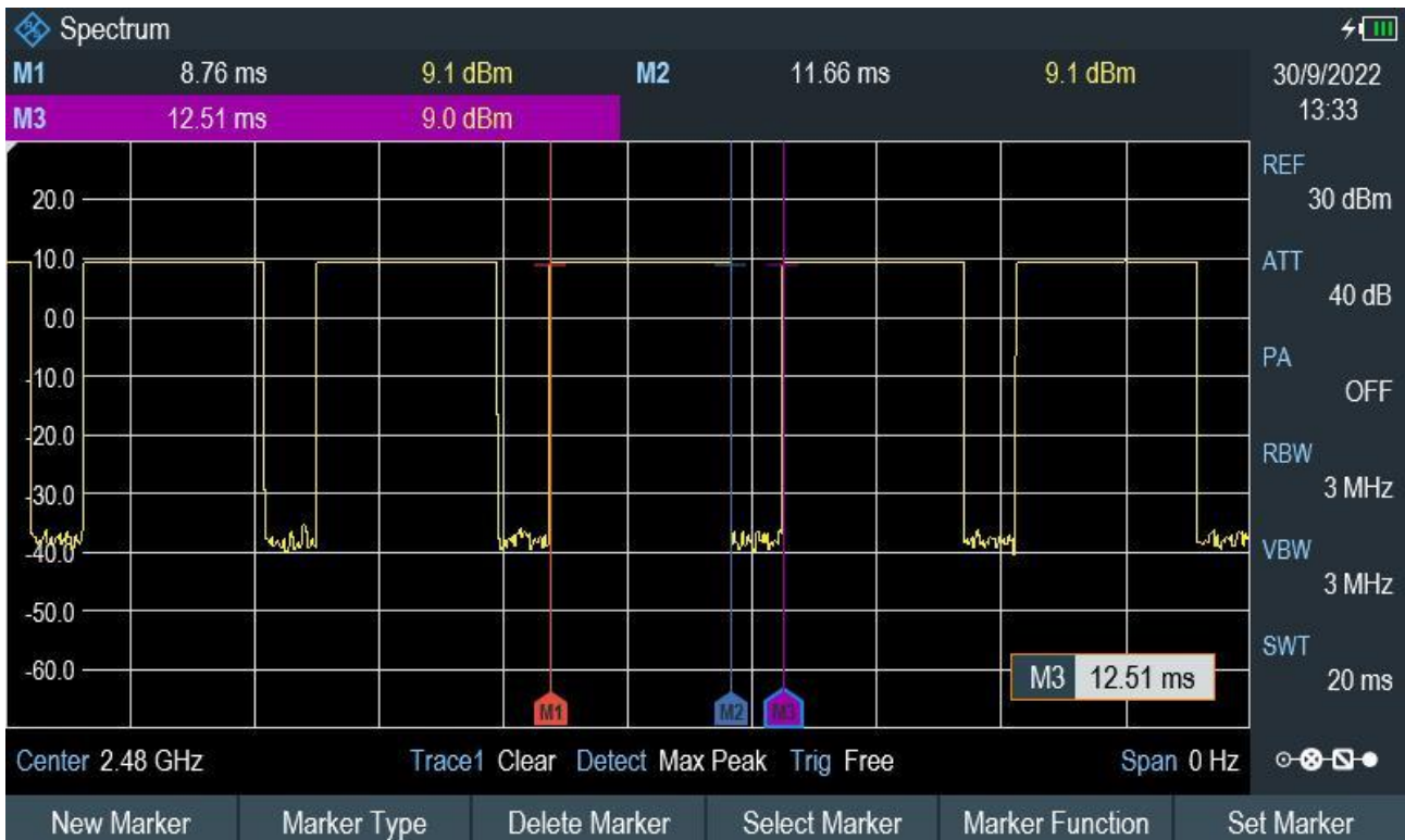
Time-domain plot for Bluetooth transmission signal
