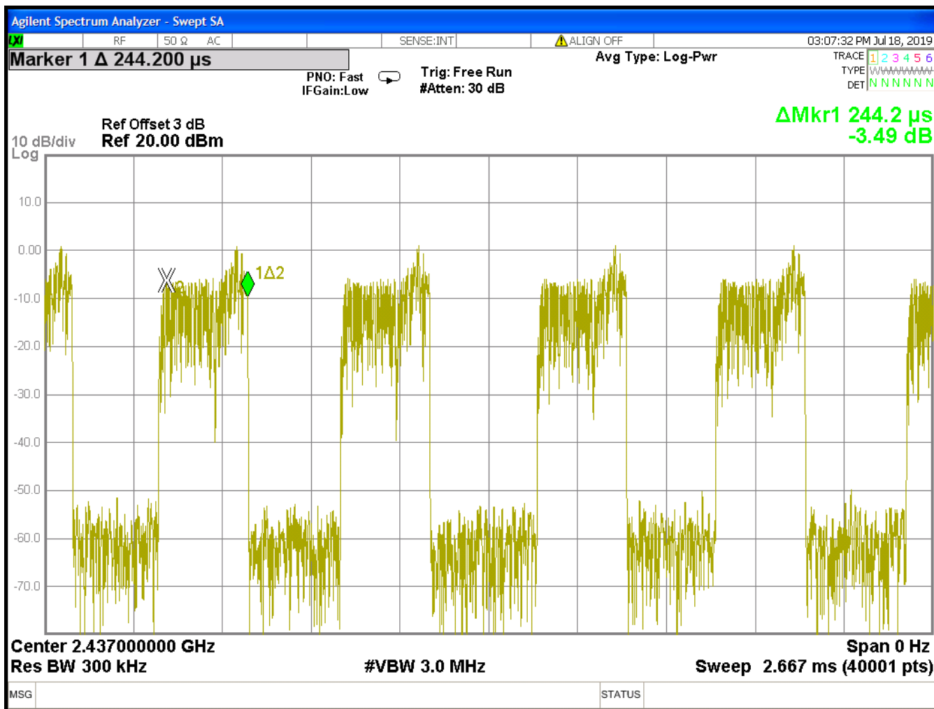
Figure 1. On Time of Transmit Pulse
