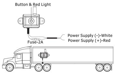
Remark: The have better performance, please install the trailer exchanger outside between the front tractor and towed trailer.
