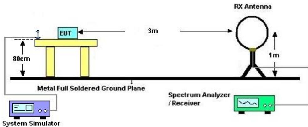
For radiated test from 30MHz to 1GHz
