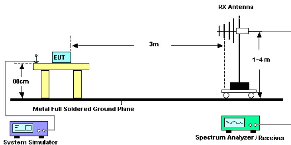
For radiated test above 1GHz
