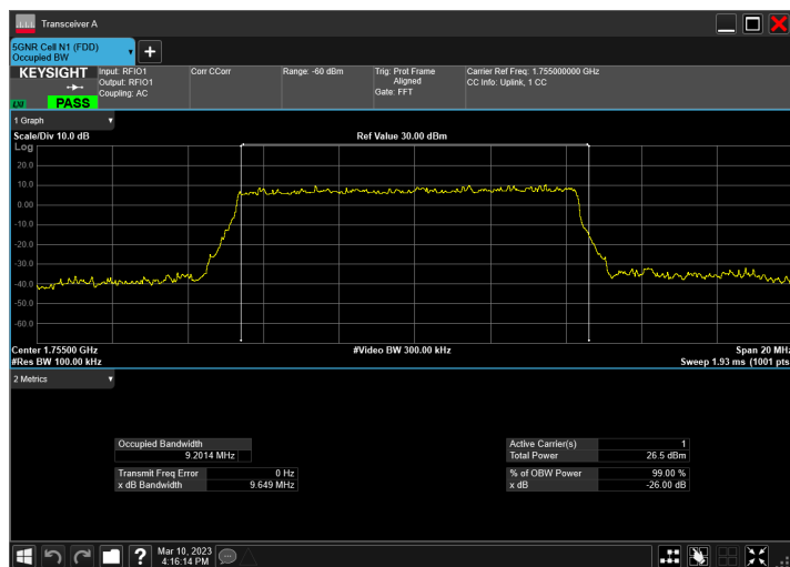
DC_5A_n66A_10MHz|10MHz_15kHz_836.5MHz|1715MHz_Q PSK|CP-OFDM 16 QAM_RB1@50|RB52@0
