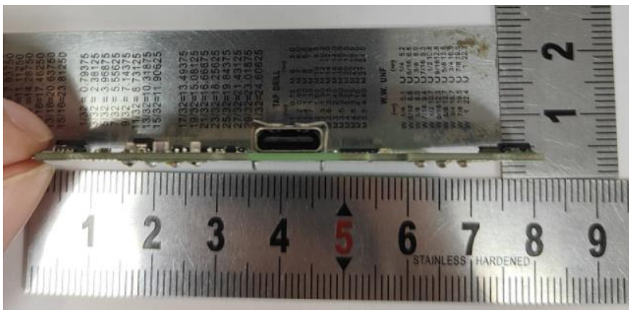
Main PCBA Front side view_ size: 73.6mm (length)*3.18mm (height)
