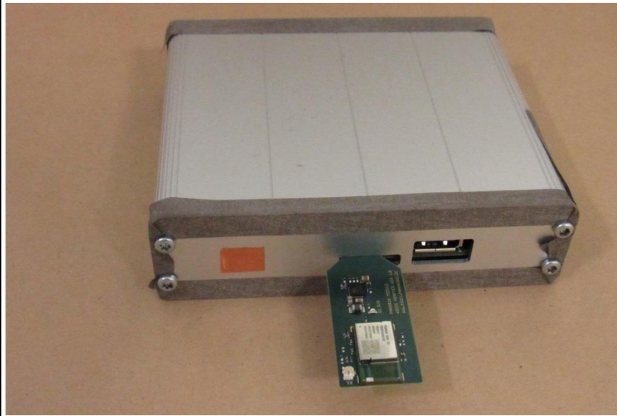
Processor board radiated, front view
