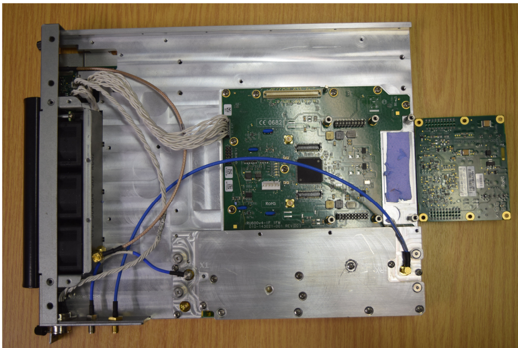
Photo 4, IRU 600v4 RFU DC power board removed:
