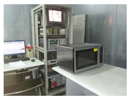
Radiated Emission Test Set-up (30 -1,000MHz):
