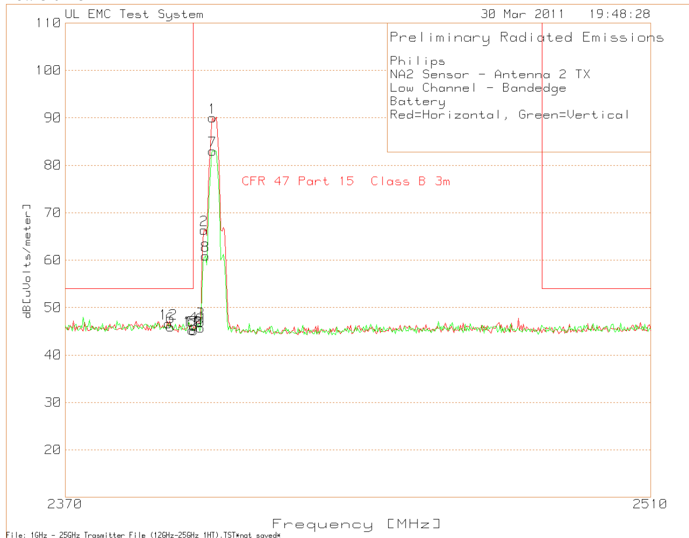
Figure 23 Radiated Band Edge Compliance Graph – Antenna 2
