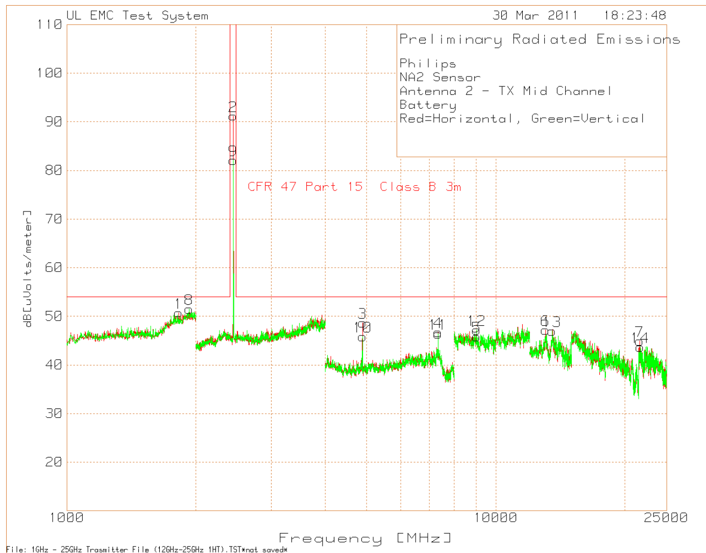
Figure 15 Radiated Spurious Emissions above 1GHz, Middle Channel – Antenna 2
